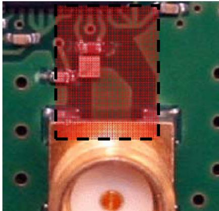
**Figure 5** Opening in power/GND planes below RF circuitry
