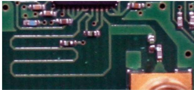
**Figure 2 Layout of transmission line implementation**
