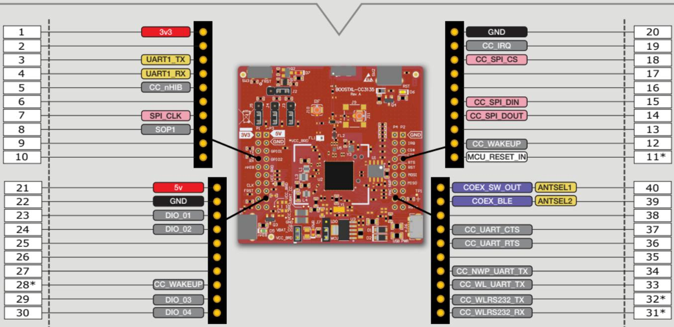
\*These pins are not connected to the Launchpad Connector by default.
