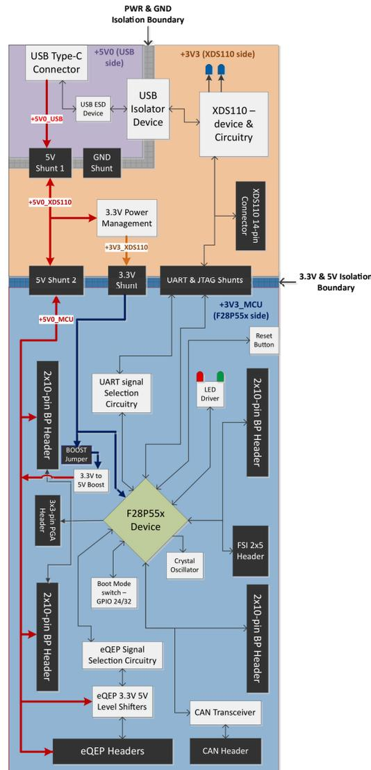
Figure 2-1. F28P55x LaunchPad Development Kit Block Diagram
