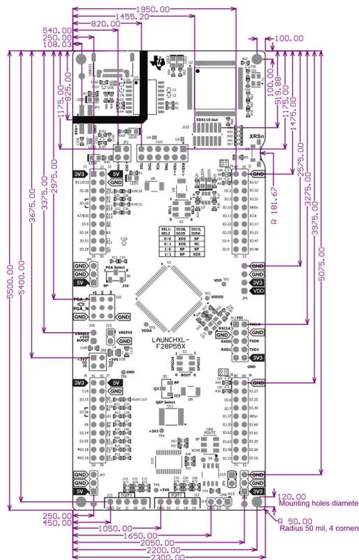
Figure 4-5. F28P55x LaunchPad Dimensions and Component Locations
