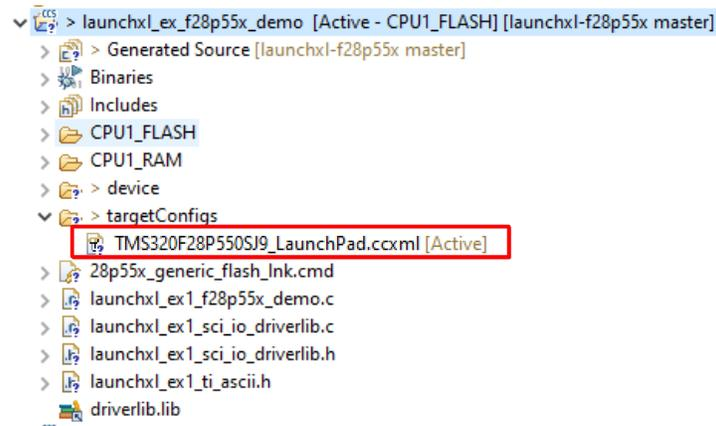
**Figure 5-2. Target Configuration Included in the Demo Project**
