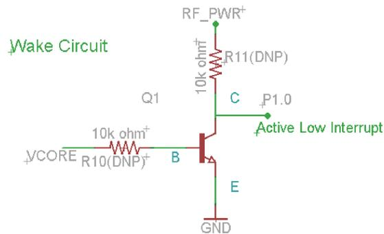
Figure 3. Wake Circuit
