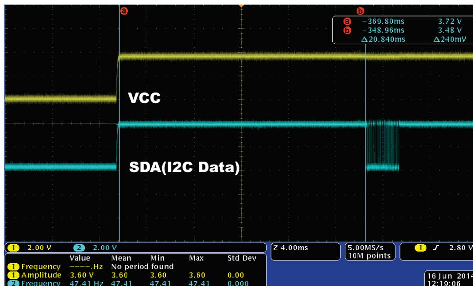
**Figure 6. Power to I2C Communication**
