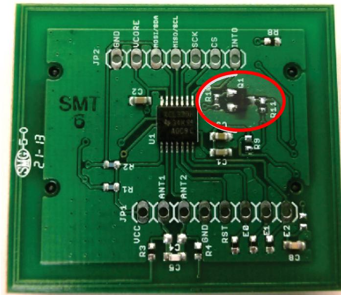
**Figure 5. RF430CL330HTB With Wake Up Circuit Populated**
