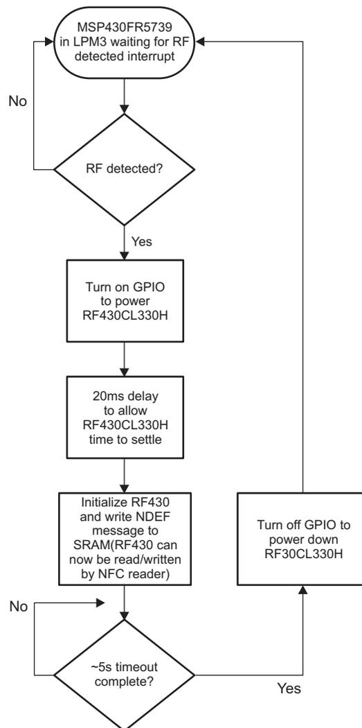
Figure 4. Typical Wake Up Operation Flow Diagram
