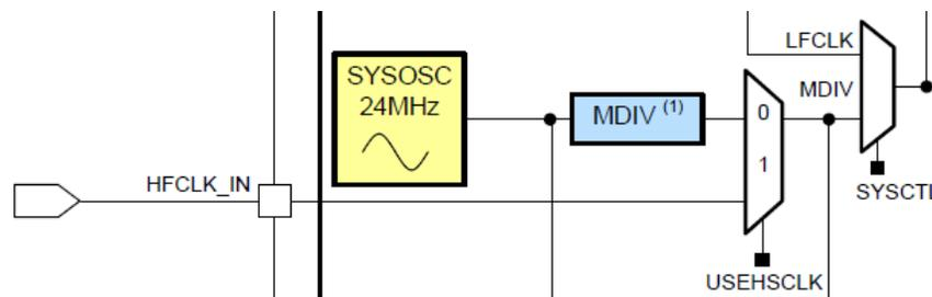
Figure 4-3. MSPM0C Series External Clock Input HFCLK\_IN
