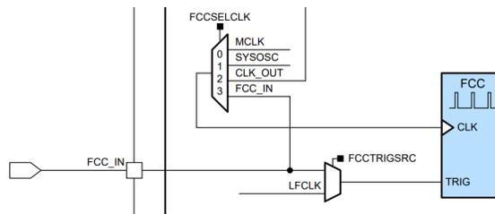
**Figure 4-5. MSPM0C Series Frequency Clock Counter Block Diagram**
