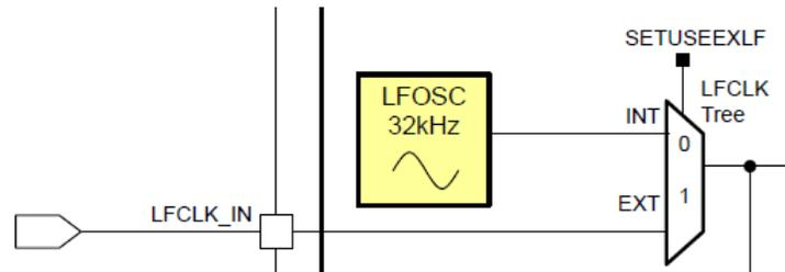
Figure 4-2. MSPM0C Series External Clock Input LFCLK\_IN
