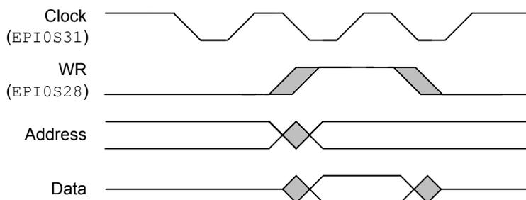
Figure 11-29. EPI Clock Operation, CLKGATE=1, WR2CYC=1
