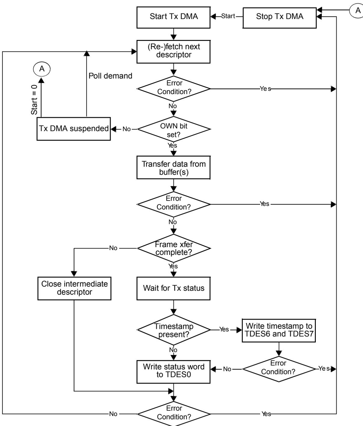
**TX DMA OSF Mode Operation**
