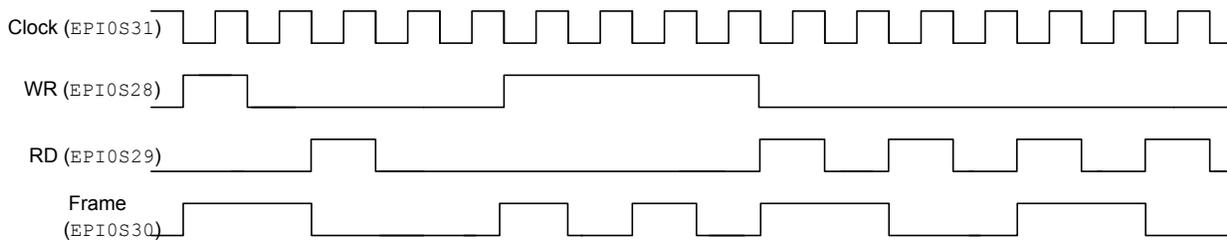
When `FRMCNT=1`, the `FRAME` signal transitions on the rising edge of the `WR` or `RD` strobes for every other access, see Figure 11-26 on page 859.
