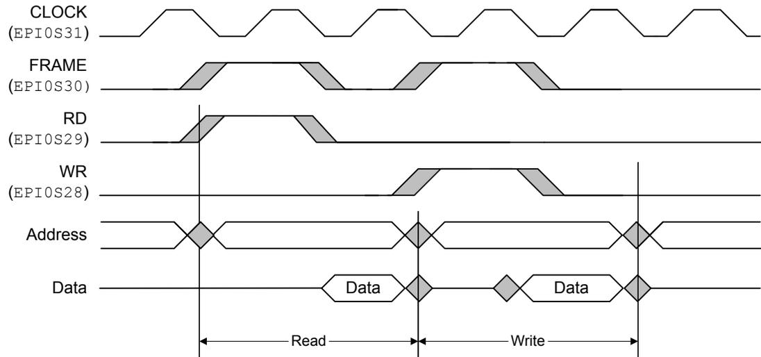
**Figure 11-21. Read Accesses, FRM50=0, FRMCNT=0**
