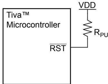
**Note:**  $R_{\text{PU}} = 0$  to 100 k $\Omega$
