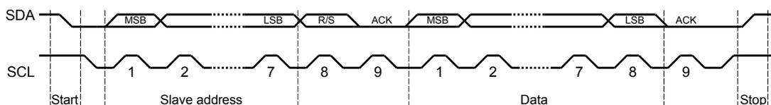
The first seven bits of the first byte make up the slave address (see Figure 21-5). The eighth bit determines the direction of the message. A zero in the R/S position of the first byte means that the master transmits (sends) data to the selected slave, and a one in this position means that the master receives data from the slave.
