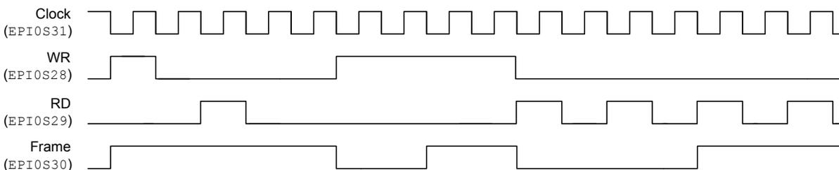
When  $FRMCNT=2$ , the FRAME signal transitions the rising edge of the WR or RD strobes for every third access, and so on for every value of  $FRMCNT$ , see Figure 11-27 on page 859.
