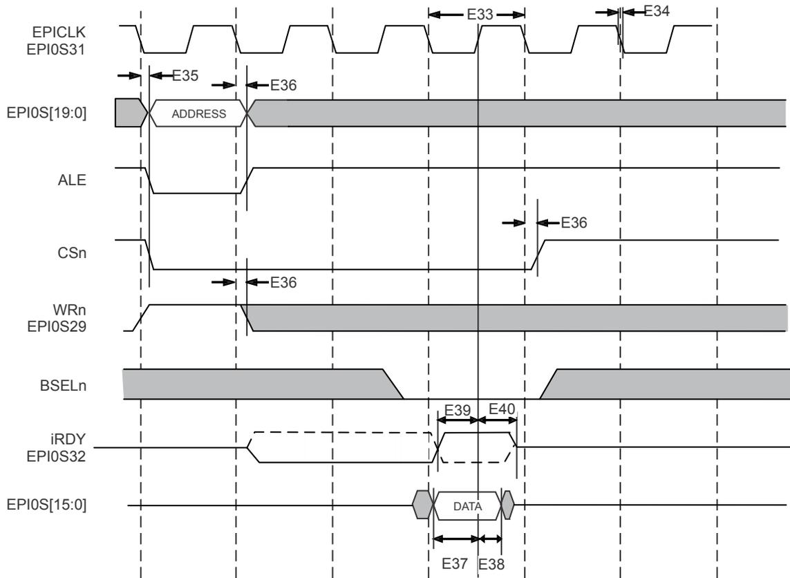
Figure 30-27. PSRAM Single Burst Write
