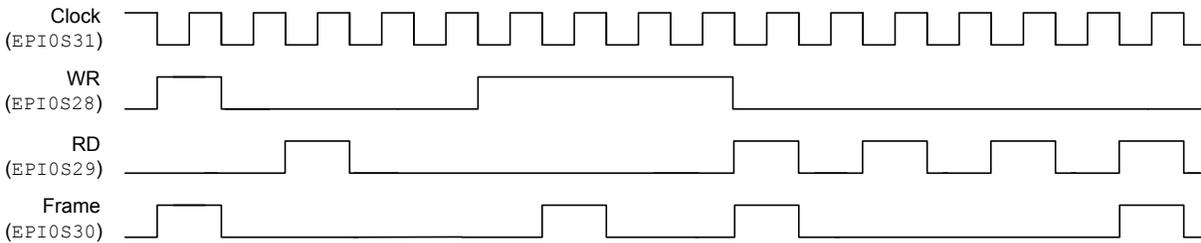
When `FRM50` is set, the `FRAME` signal transitions on the rising edge of either the `WR` or `RD` strobes. When `FRMCNT=0`, the `FRAME` signal transitions on the rising edge of `WR` or `RD` for every access, see Figure 11-25 on page 858.
