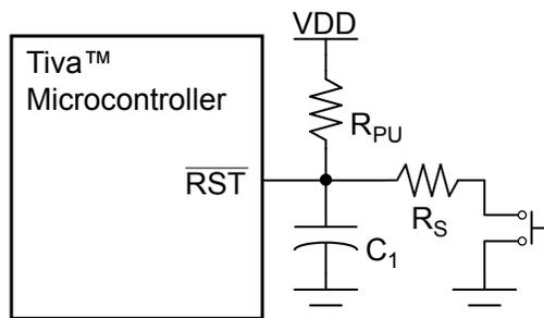
**Note:** Typical  $R_{\text{PU}} = 10$  k $\Omega$
