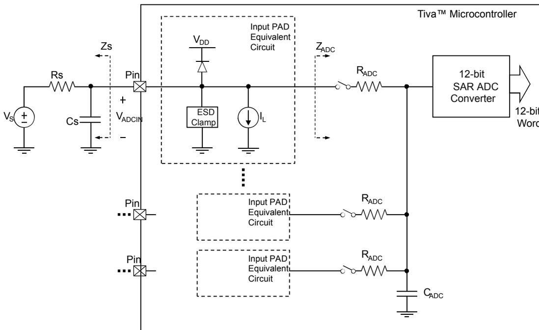
The ADC operates from both the 3.3-V analog and 1.2-V digital power supplies. The ADC clock can be configured to reduce power consumption when ADC conversions are not required (see “System Control” on page 245). The analog inputs are connected to the ADC through specially balanced input paths to minimize the distortion and cross-talk on the inputs. Detailed information on the ADC power supplies and analog inputs can be found in “Analog-to-Digital Converter (ADC)” on page 1938.
