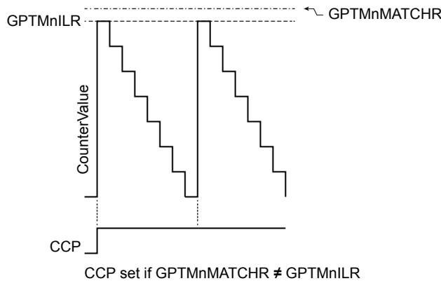
Figure 16-6 on page 1091 shows how the CCP output operates when the  $PLO$  and  $MRSU$  bits are set and the **GPTMTnMATCHR** value is the same as the **GPTMTnILR** value. In this situation, if the  $PLO$  bit is 0, the CCP signal goes high when the **GPTMTnILR** value is loaded and the match would be essentially ignored.
