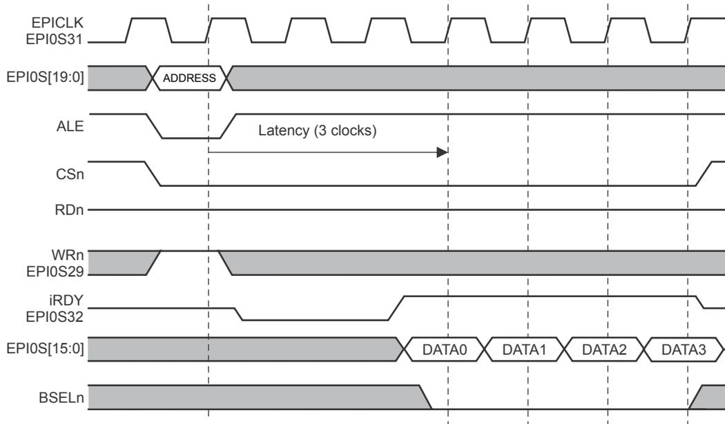
Figure 11-8. PSRAM Burst Write
