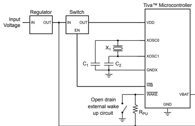
**Note:** Some devices may not supply a `GNDX` signal. See “Signal Tables” on page 1833 for pins specific to your device.
