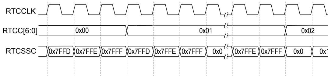
In the case of a trim value below 0x7FFF, the RTCSSC value is advanced from 0x7FFF to the trim value while the RTCC value is incremented from 0x0 to 0x1. If the match value is within that range, the match interrupt is not triggered. For example, as shown in Figure 7-6 on page 545, if the match interrupt was configured with RTCM0=0x1 and RTCSSM=0x2, an interrupt would never be triggered.
