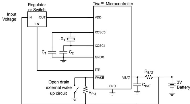
**Note:** Some devices may not supply the GNDX signal. If GNDX is absent, the crystal load capacitors can be tied to GND externally. See “Signal Tables” on page 1833 for pins specific to your device.
