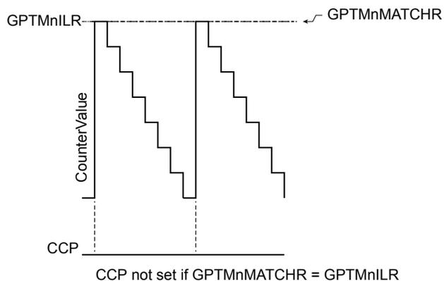
Figure 16-7 on page 1091 shows how the CCP output operates when the `PLO` and `MRSU` bits are set and the `GPTMTnILR` is greater than the `GPTMTnMATCHR` value.
