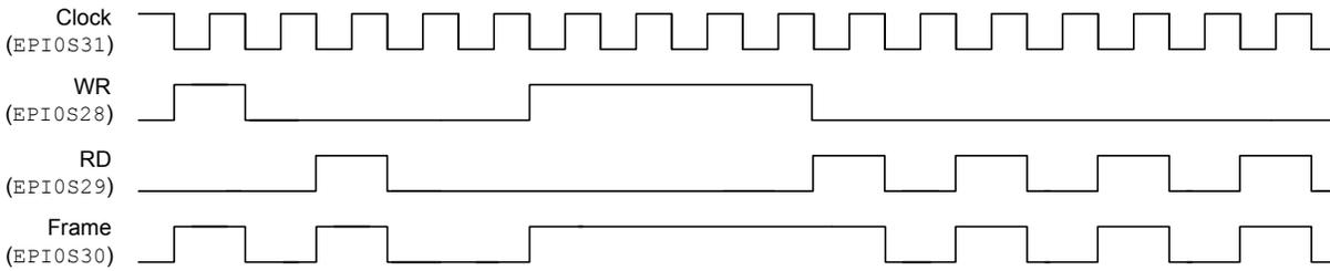
If the `FRMCNT` field is `0x1`, then the `FRAME` signal pulses high during every other read or write access, see Figure 11-23 on page 858.
