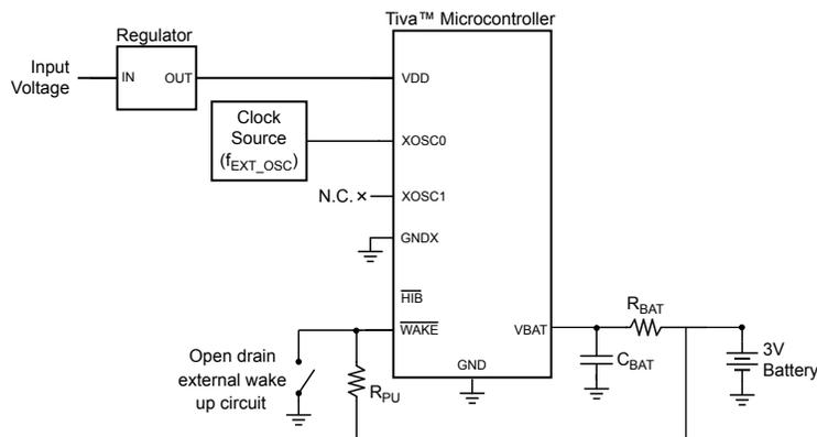
**Note:** Some devices may not supply a GNDX signal. See “Signal Tables” on page 1833 for pins specific to your device.
