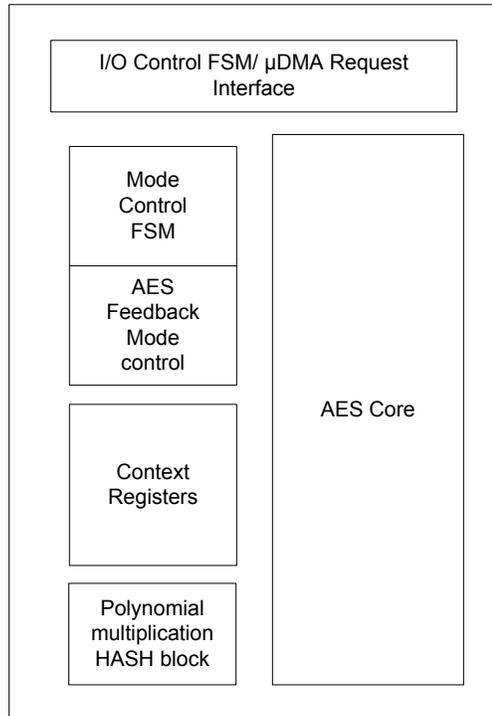
AES is an efficient implementation of the Rijndael cipher (the AES algorithm) and a 128-bit polynomial multiplication (referred to here as GHASH, as per the AES-GCM specification). Rijndael is a block cipher in which each data block is 128 bits. The polynomial multiplication multiplies two 128-bit vectors using the smallest 128-bit irreducible polynomial, represented by the following 128-bit string:  $\{0^{120}\}||10000111$ . The two implementations are combined into the AES wide-bus engine.
