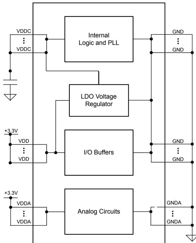
**Note:** The  $V_{DDA}$  voltage source is typically connected to a filtered voltage source or regulator.
