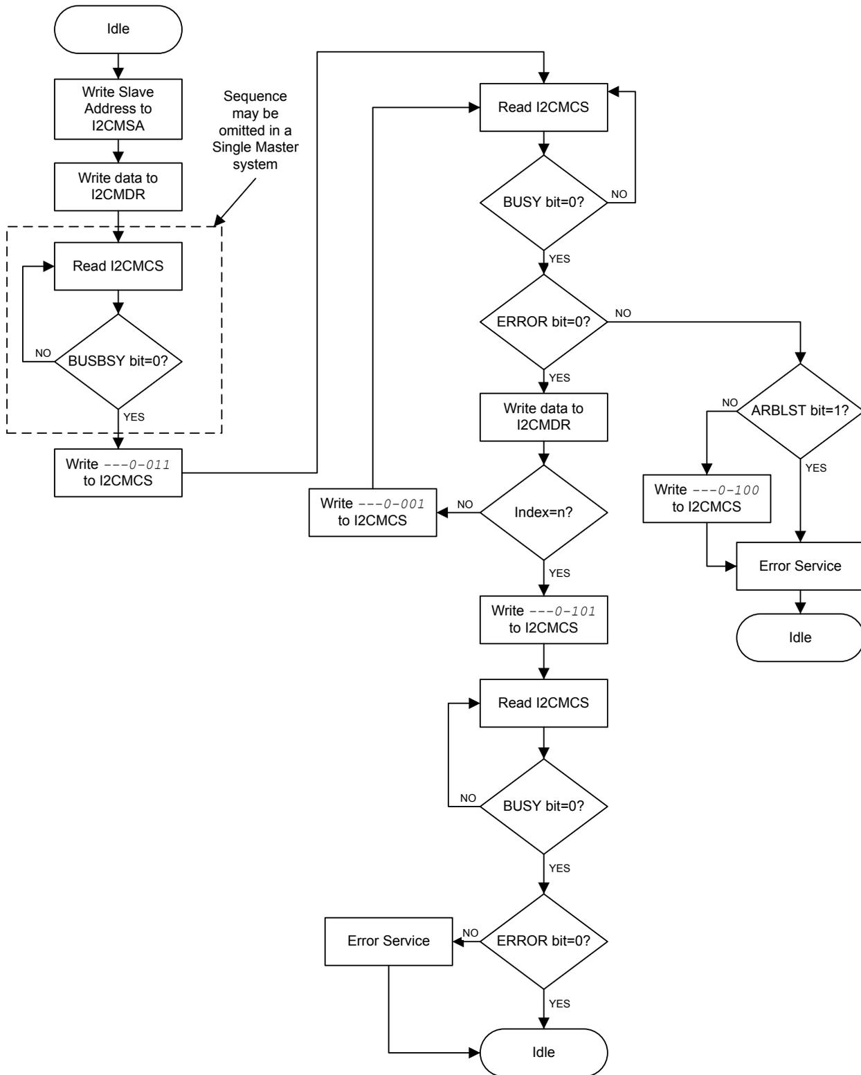
Figure 21-11. Master RECEIVE of Multiple Data Bytes
