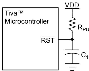
**Note:**  $R_{\text{PU}} = 1$  k $\Omega$  to 100 k $\Omega$
