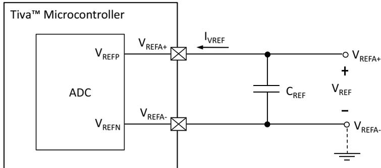
**Figure 30-29. ADC Input Equivalency**
