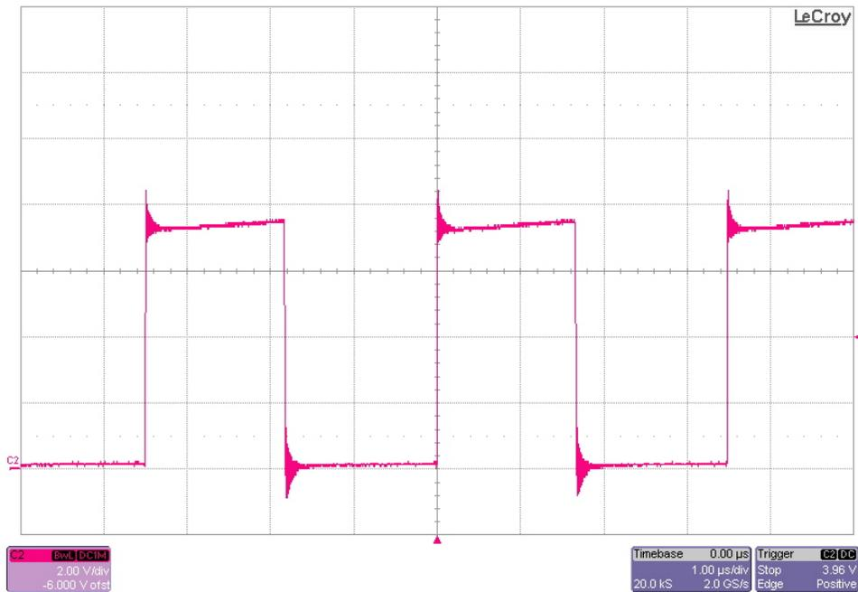
The photo below shows the FET switching voltage. The input voltage is 3.0V and the output is loaded to 0.35A. The converter is operating in DCM. (2V/DIV, 1uS/DIV)
