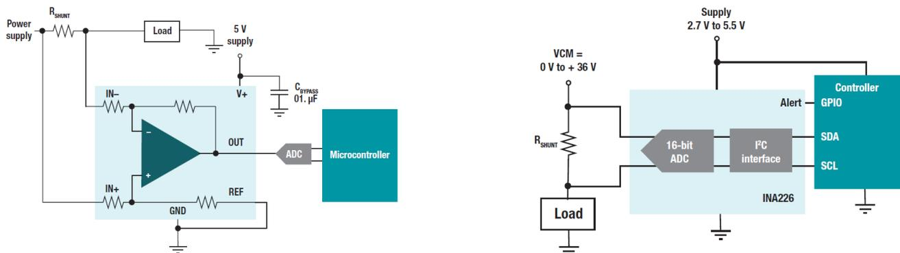
**Figure 2. Analog vs. Digital Output Current Sense Amplifiers**
