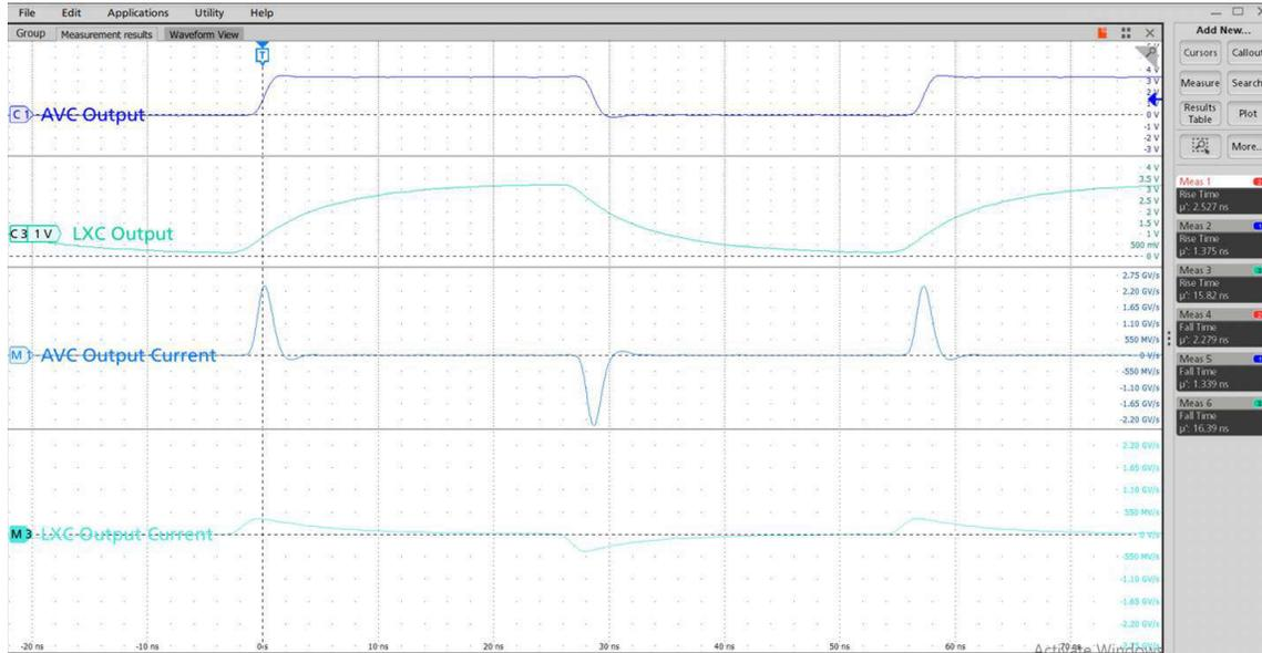
**Figure 4-4. Transient Switching Current for SN74AVCxT245 and SN74LXCxT245**
