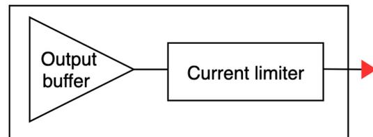
Figure 4-2. High DC Drive Strength Buffer With Transient Current Limiter Circuit (LXC)
