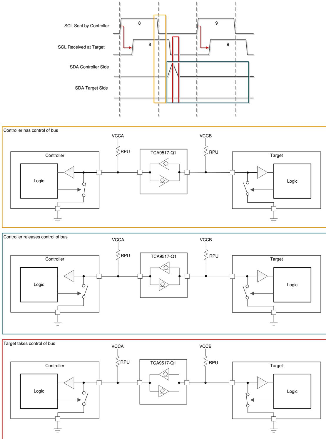
**Figure 3-3. SDA Handoff Delay Illustration**
