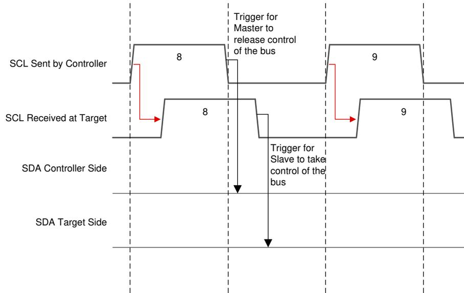
**Figure 3-2. Eighth to Ninth Clock Cycle Zoomed in With Propagation Delay From Buffer**
