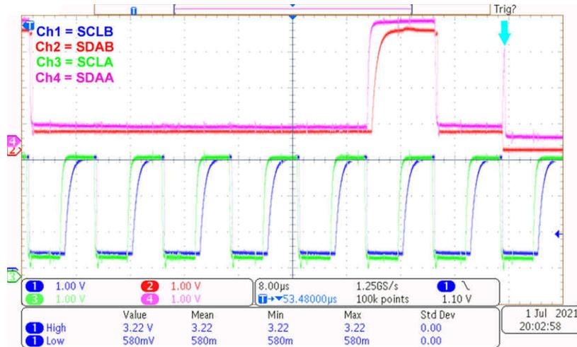
Figure 3-5. SDA Handoff Delay With Nine Clock Pulses
