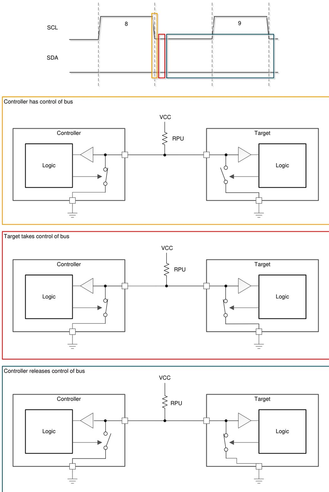
**Figure 2-2. I<sup>2</sup>C SDA Handoff With Overlap**
