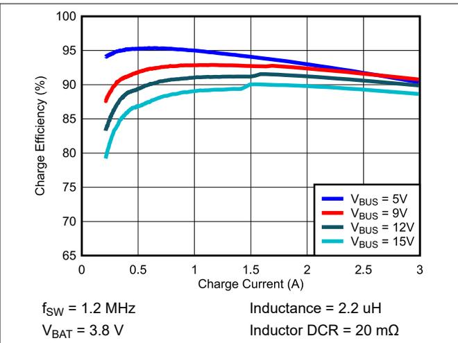
Figure 7-2. 1-Cell Battery Charge Efficiency vs Charge Current
