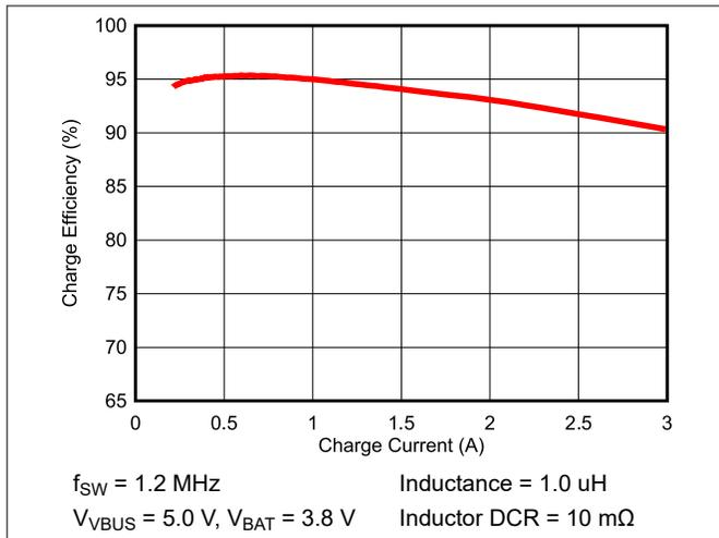
Figure 7-1. 1-Cell Battery Charge Efficiency vs Charge Current
