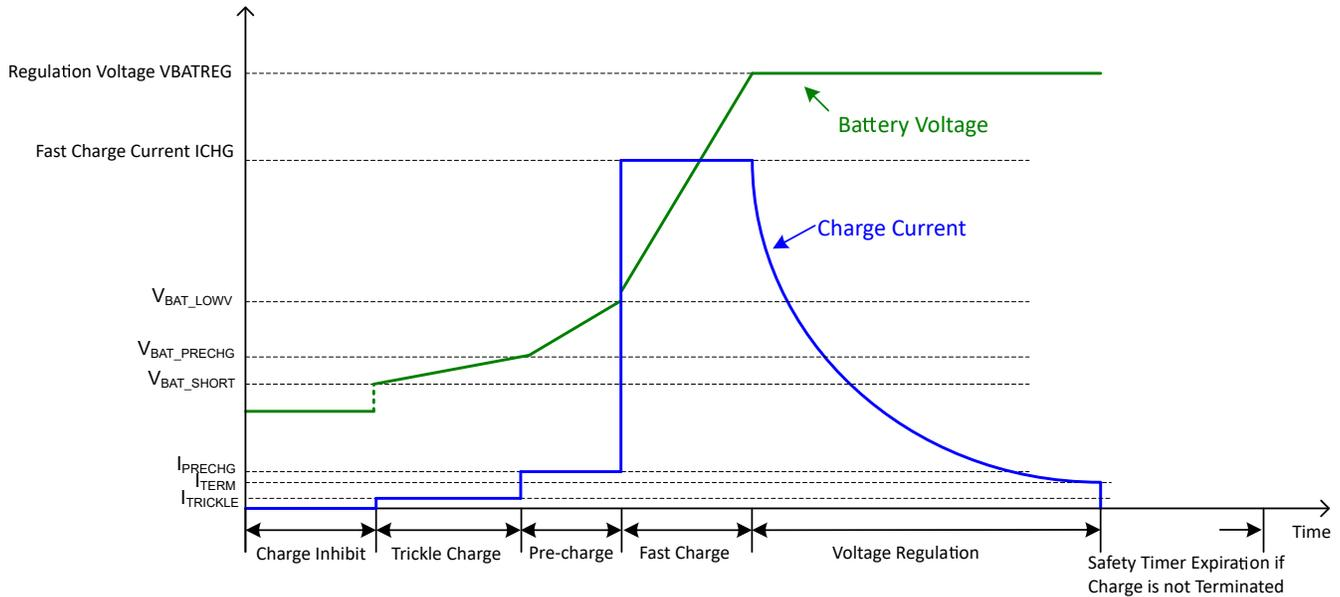
Figure 8-2. Battery Charging Profile for  $V_{BATREG} = 3.6V$
