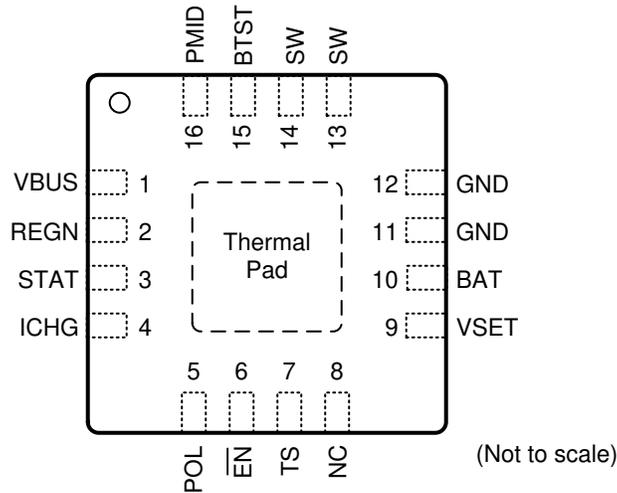
Figure 6-1. RTE Package 16-Pin WQFN Top View
