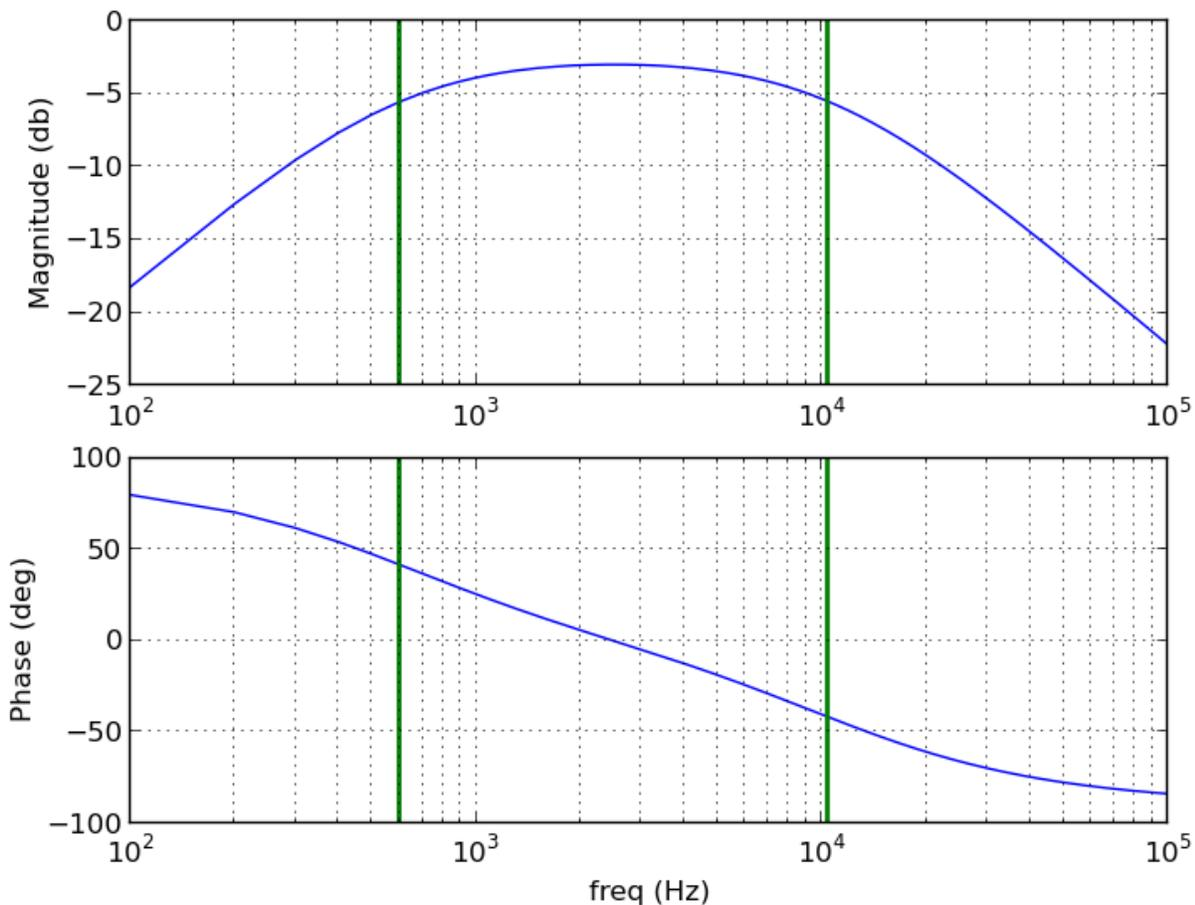
图 8. Band-Pass Filter and Frequency Response
