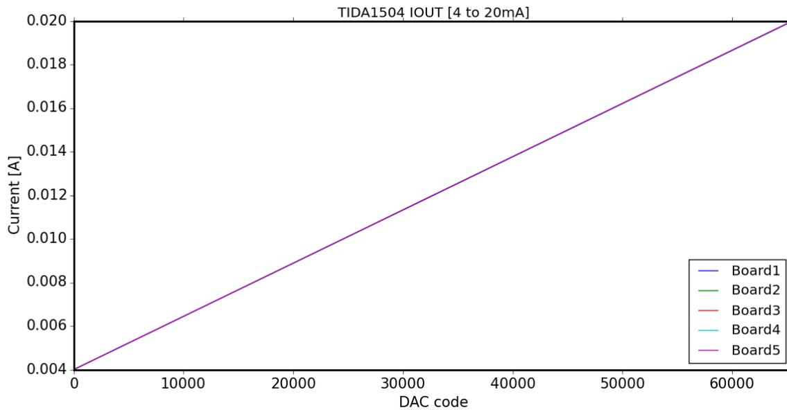
图 11. Measured Transfer Function
