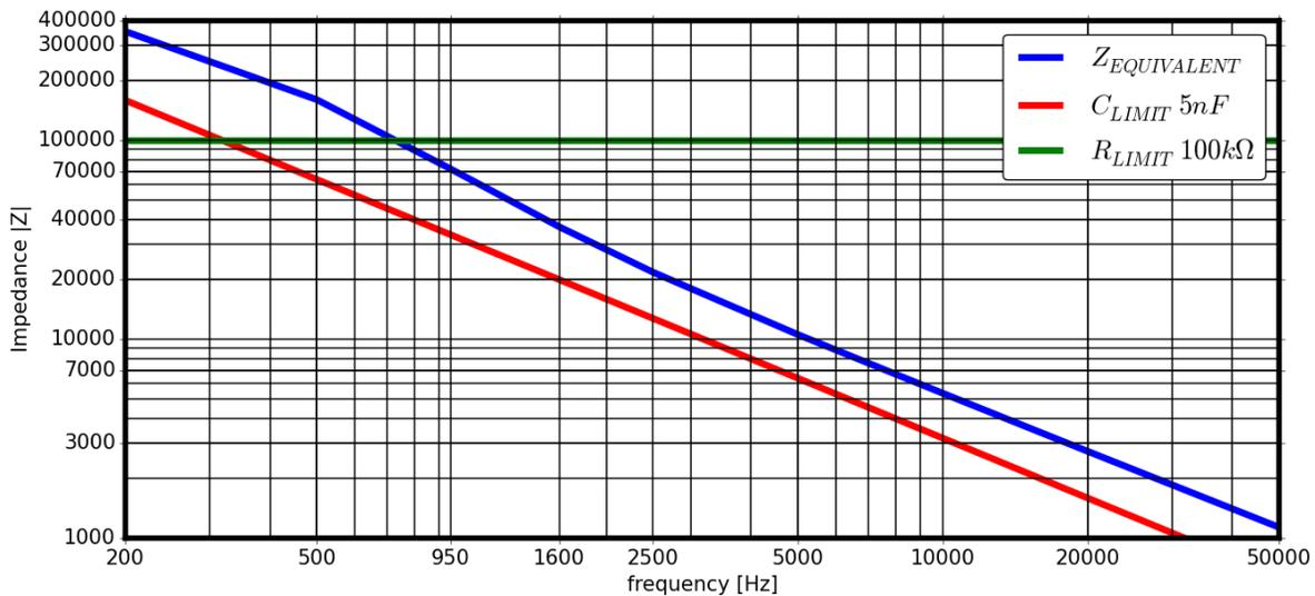
图 20. Impedance of Design versus Frequency
