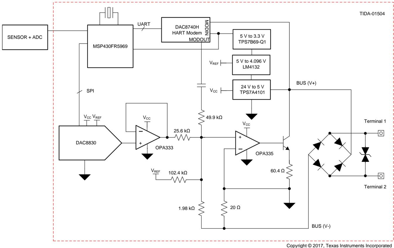
图 1. Detailed Circuit Diagram of TIDA-01504
