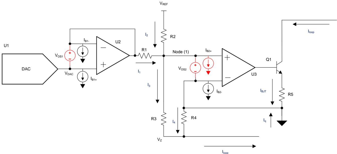
图 6. Transmitter V/I With Error Sources
