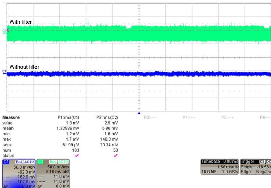
图 17. Output Noise During Silence Measurement
