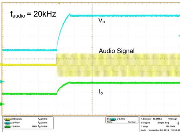
Figure 6.1 Output Voltage Transition at  $f_{audio}=20kHz$
