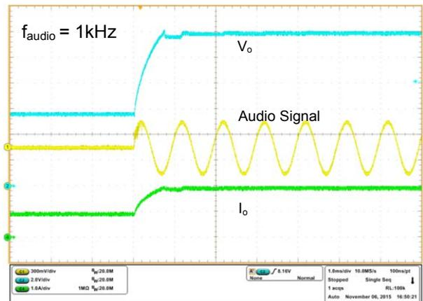
Figure 6.2 Output Voltage Transition at  $f_{audio}=1kHz$
