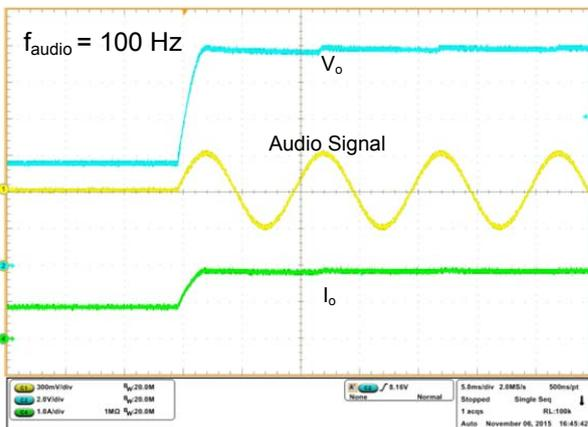
Figure 6.3 Output Voltage Transition at  $f_{audio}=100Hz$
