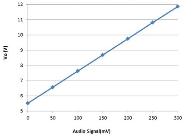
Figure 5  $V_o$  VS. Audio Signal
