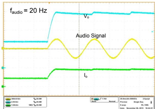
Figure 6.4 Output Voltage Transition at  $f_{audio}=20Hz$
