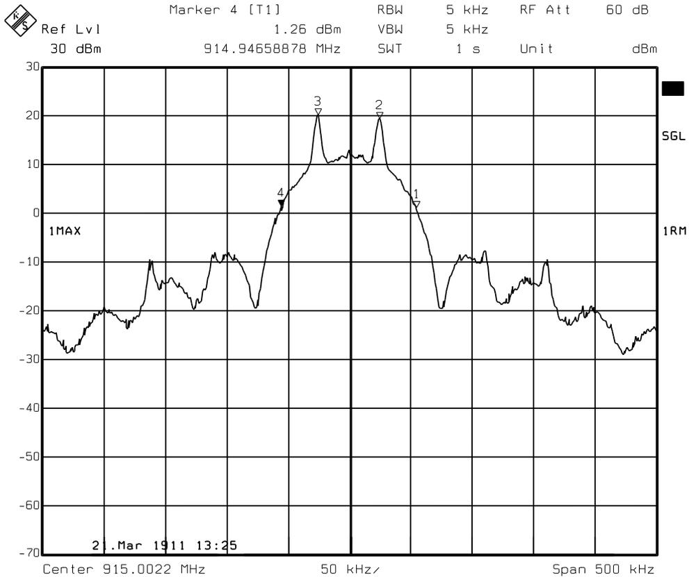
**Figure 4.16. Typical Modulation Bandwidth, 50 kbps, PATABLE = 0x80. Measured according to FCC 15.247**
