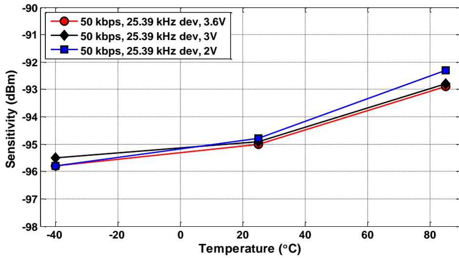
Figure 4.5. Typical Sensitivity vs. Temperature and Power Supply Voltage, LGM, 50 kbps
