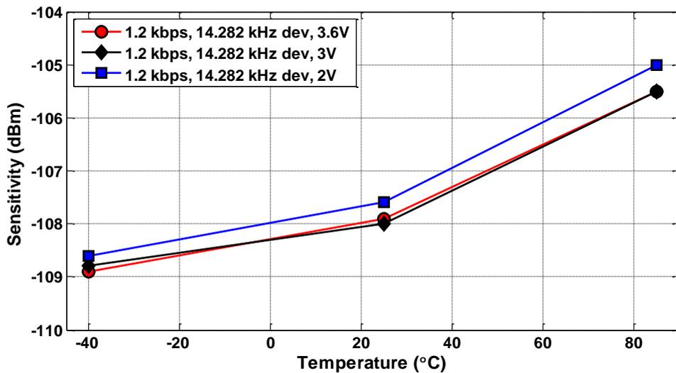
Figure 4.4. Typical Sensitivity vs. Temperature and Power Supply Voltage, LGM, 1.2 kbps
