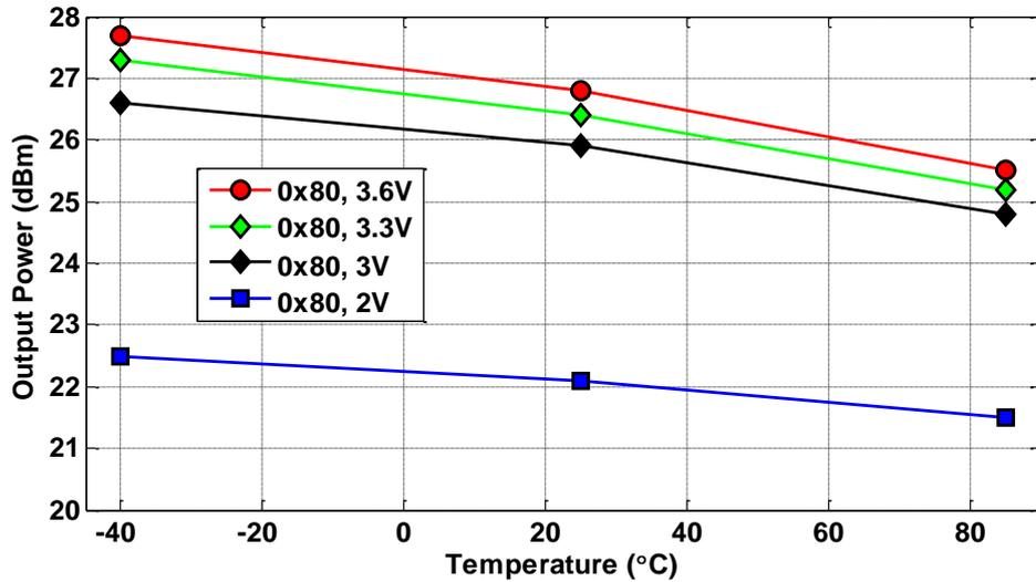
Figure 4.12. Typical Output Power vs. Temperature and Power Supply Voltage. PATABLE = 0x80
