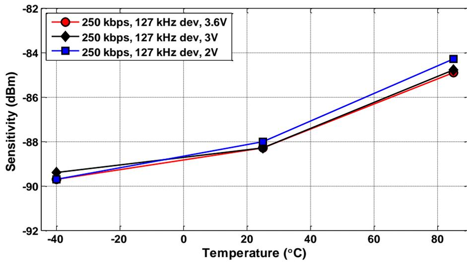
Figure 4.6. Typical Sensitivity vs. Temperature and Power Supply Voltage, LGM, 250 kbps
