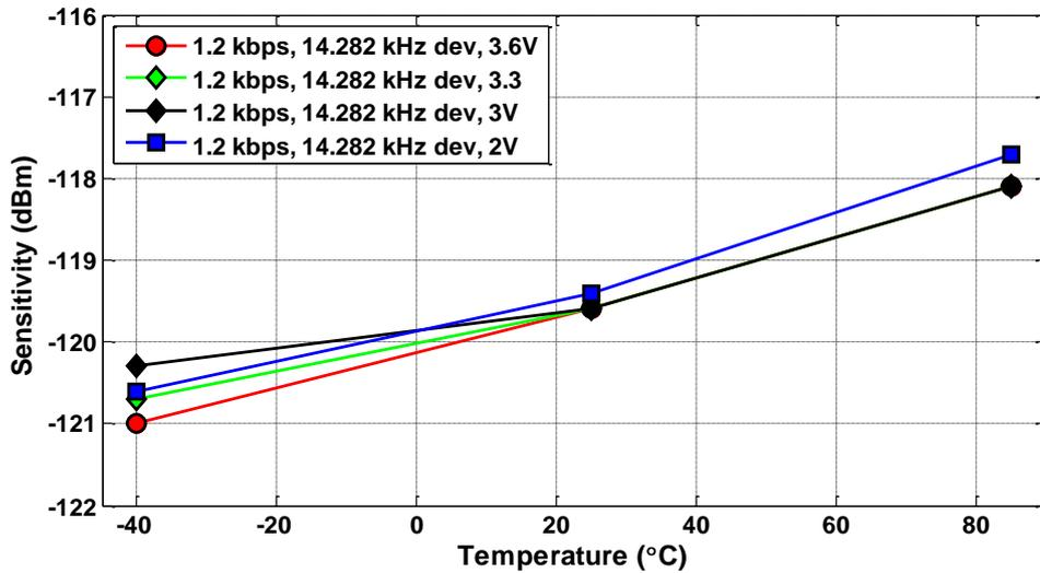
Figure 4.1. Typical Sensitivity vs. Temperature and Power Supply Voltage, HGM, 1.2 kbps
