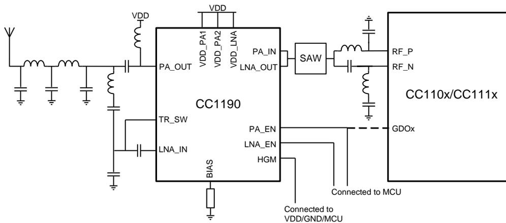
Figure 5.1. Simplified CC11xx-CC1190 Application Circuit
