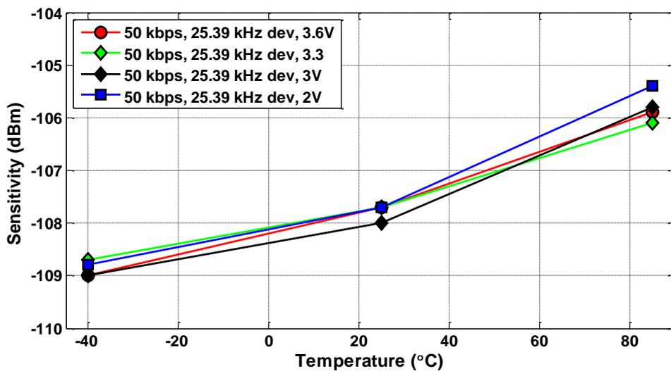
Figure 4.2. Typical Sensitivity vs. Temperature and Power Supply Voltage, HGM, 50 kbps
