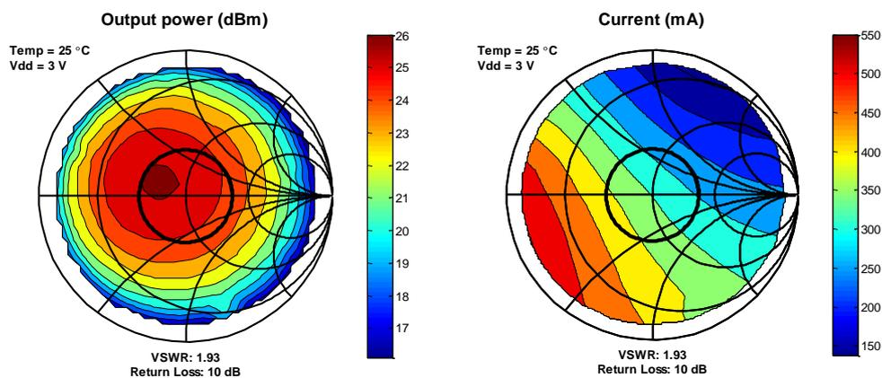
**Figure 4.18. Output Power (left) and Current (right) vs. Load Impedance at SMA Connector at 25°C. PATABLE = 0x80.**
