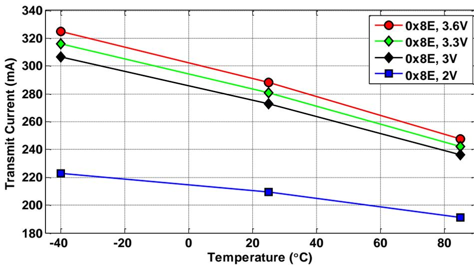
Figure 4.15. Typical TX Current Consumption vs. Temperature and Power Supply Voltage.
