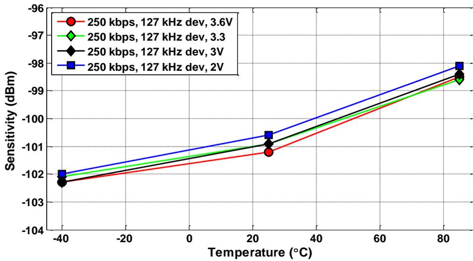
Figure 4.3. Typical Sensitivity vs. Temperature and Power Supply Voltage, HGM, 250 kbps
