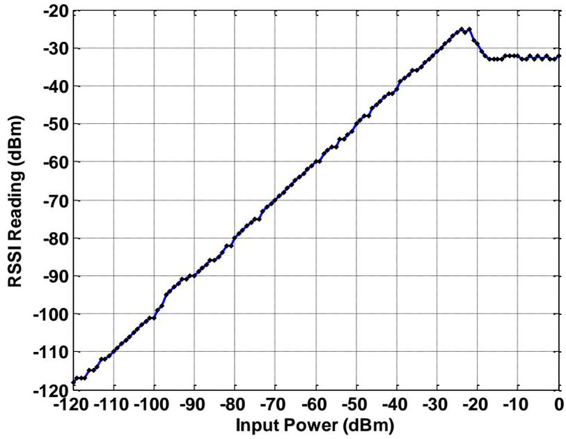
Figure 4.10. Typical RSSI vs. Input Power Level, HGM, 50 kbps
