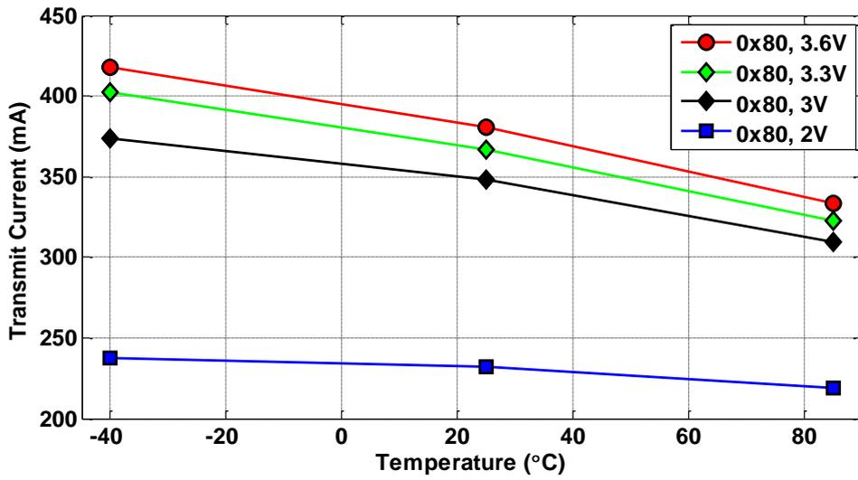
Figure 4.14. Typical TX Current Consumption vs. Temperature and Power Supply Voltage.
