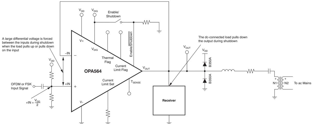
**Figure 1. Unity-Gain Powerline Communications Line Driver with DC-Coupled Load**
