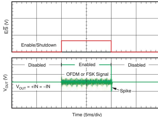
Figure 5. Output Results for Properly Configured Circuit (AC Load Only)
