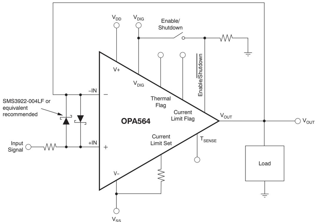
Figure 8. Dual Supply, DC-Connected Load Unity-Gain Follower
