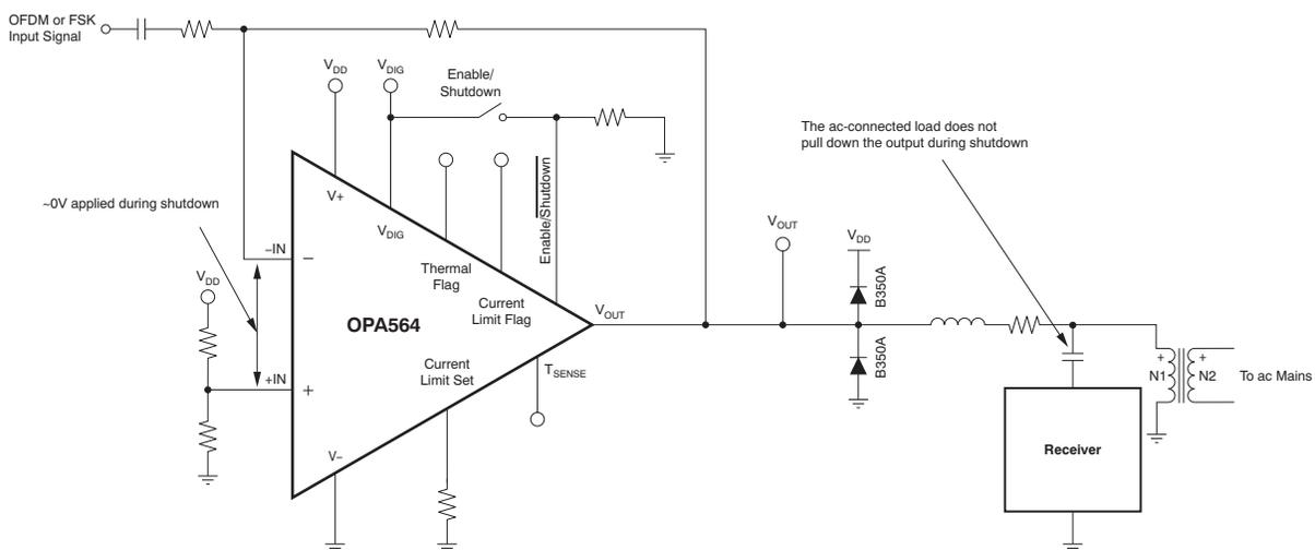
Figure 4. AC-Coupled, Inverting Gain Powerline Communications Line Driver with AC-Coupled Load
