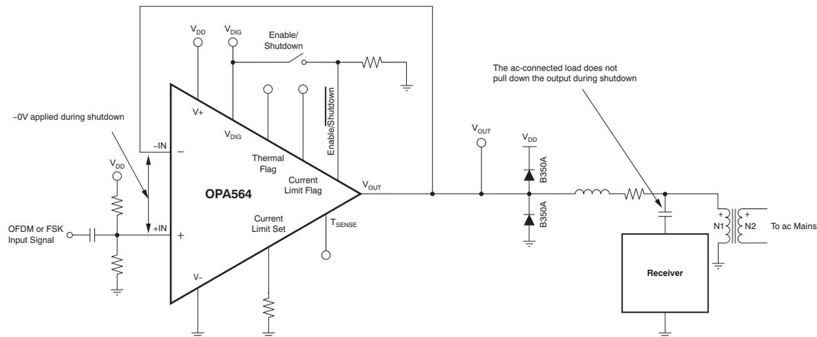
Figure 3. Unity-Gain Powerline Communications Line Driver with AC-Coupled Load
