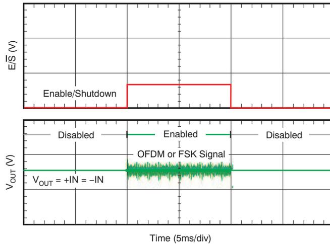
Figure 7. Output Results for Properly Configured Circuit with Voltage Divider
