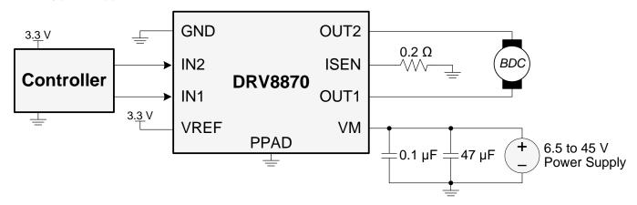
Figure 7. Typical Connections
