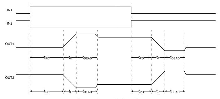
Figure 6. Propagation Delay Time
