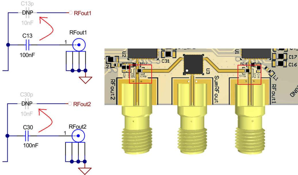
**Figure 7-1. EVM Modification for Phase Noise Reduction**
