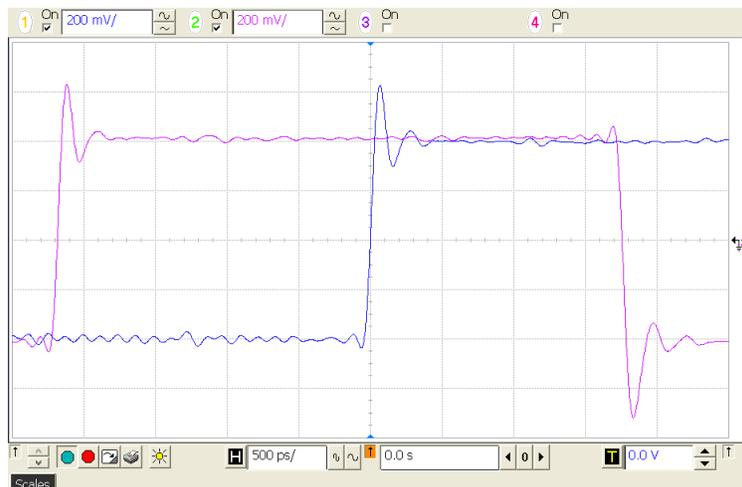
Figure 3-2. Output Phases Before Synchronization
