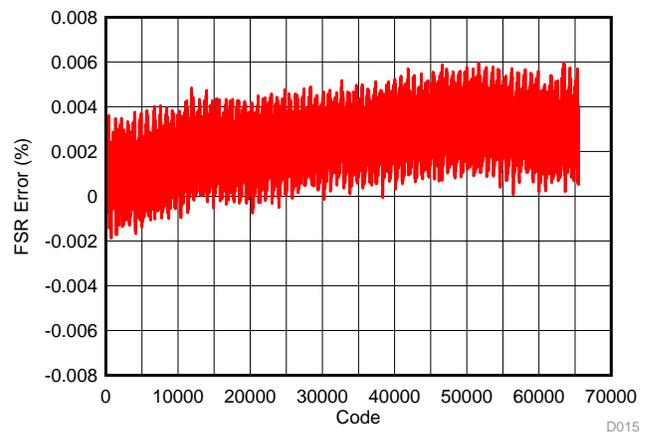
Figure 26. ±10-V Range, Code versus FSR Error (%) After Calibration
