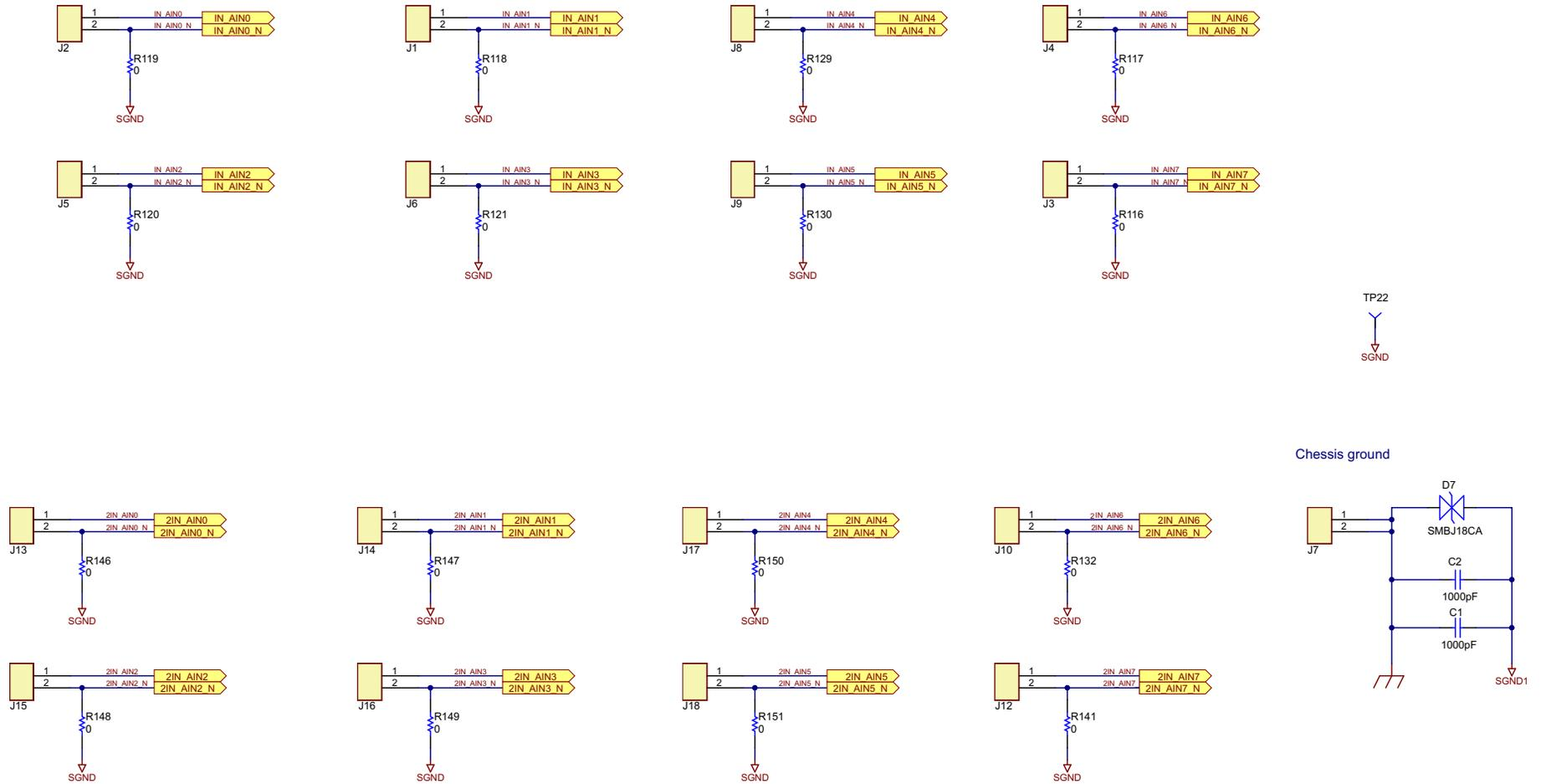
Figure 30. ADC<sub>1</sub> and ADC<sub>2</sub> Inputs Schematic
