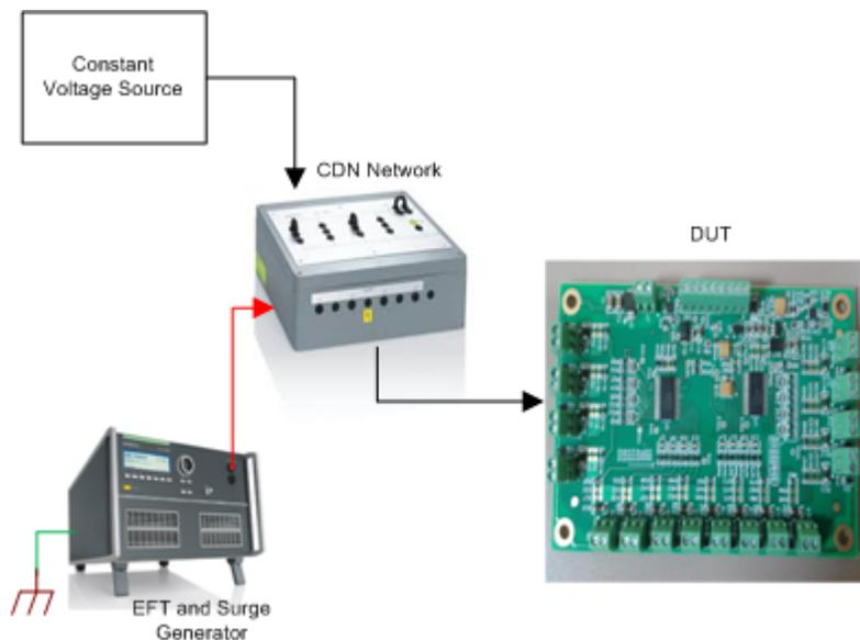
**Figure 28. Surge Test Setup**
