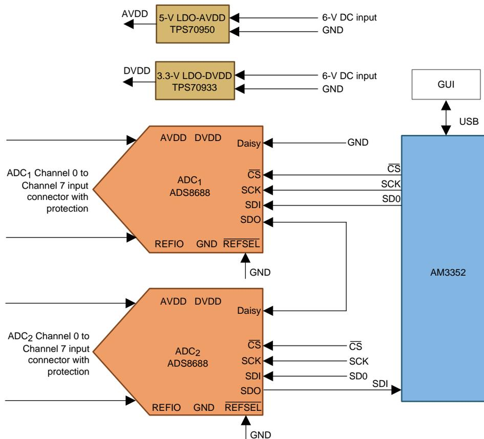
**Figure 1. System Block Diagram for TIDA-00307**
