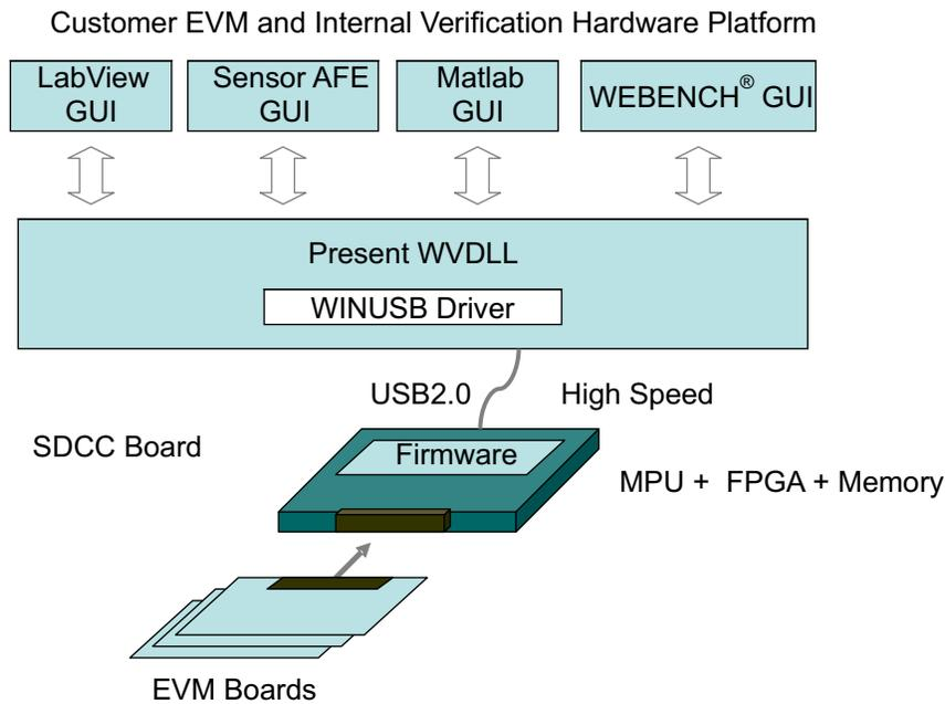
Figure 19. GUI to Capture ADC Data
