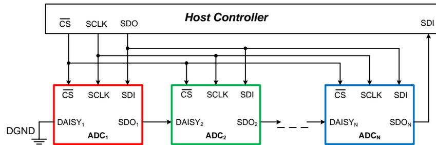
Figure 7. Daisy-Chain Diagram
