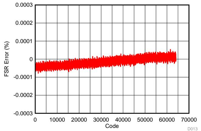
Figure 24. 0 to 10-V Range, Code versus FSR Error (%) After Calibration
