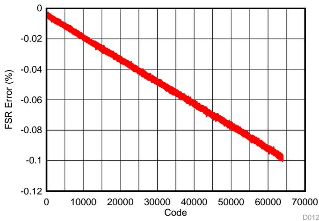
Figure 23. 0 to 10-V Range, Code versus FSR Error (%) Before Calibration
