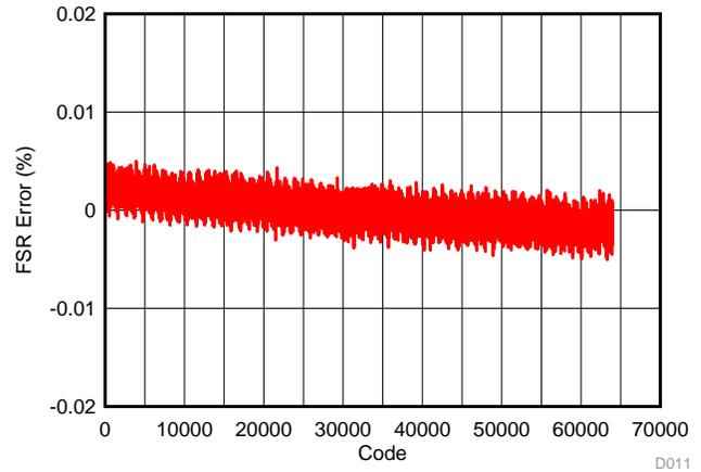
Figure 22. 0 to 5-V Range, Code versus FSR Error (%) After Calibration
