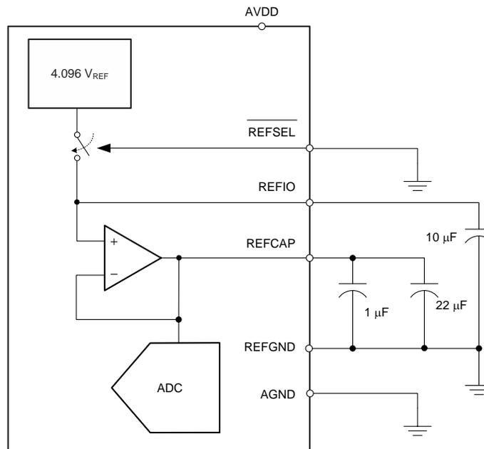
Figure 5. ADS8688 Connections for Using an Internal 4.096-V Reference
