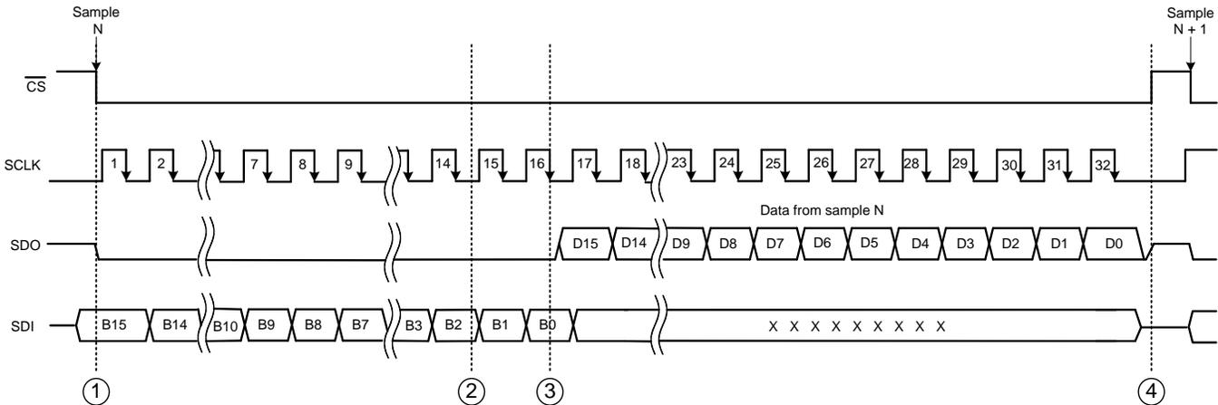
**Figure 16. Device Operation Using the Serial Interface Timing Diagram**
