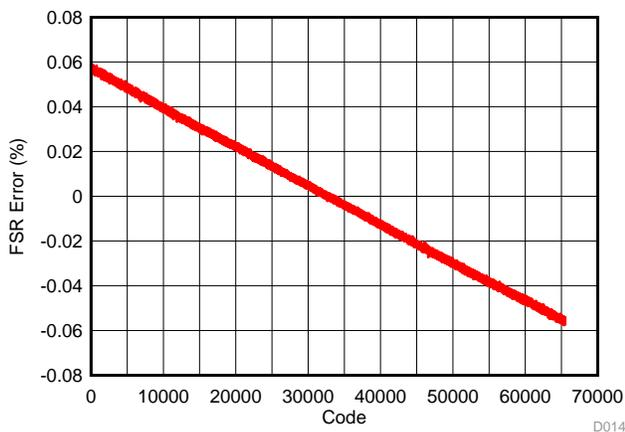
Figure 25. ±10-V Range, Code versus FSR Error (%) Before Calibration
