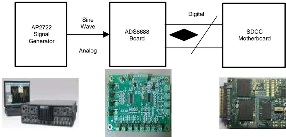
Figure 20. ADC Measurement Setup
