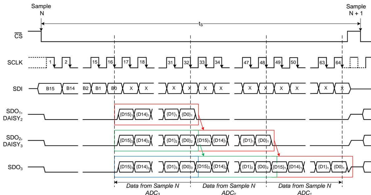
Figure 8. Timing Diagram for Devices Connected in Daisy-Chain Mode
