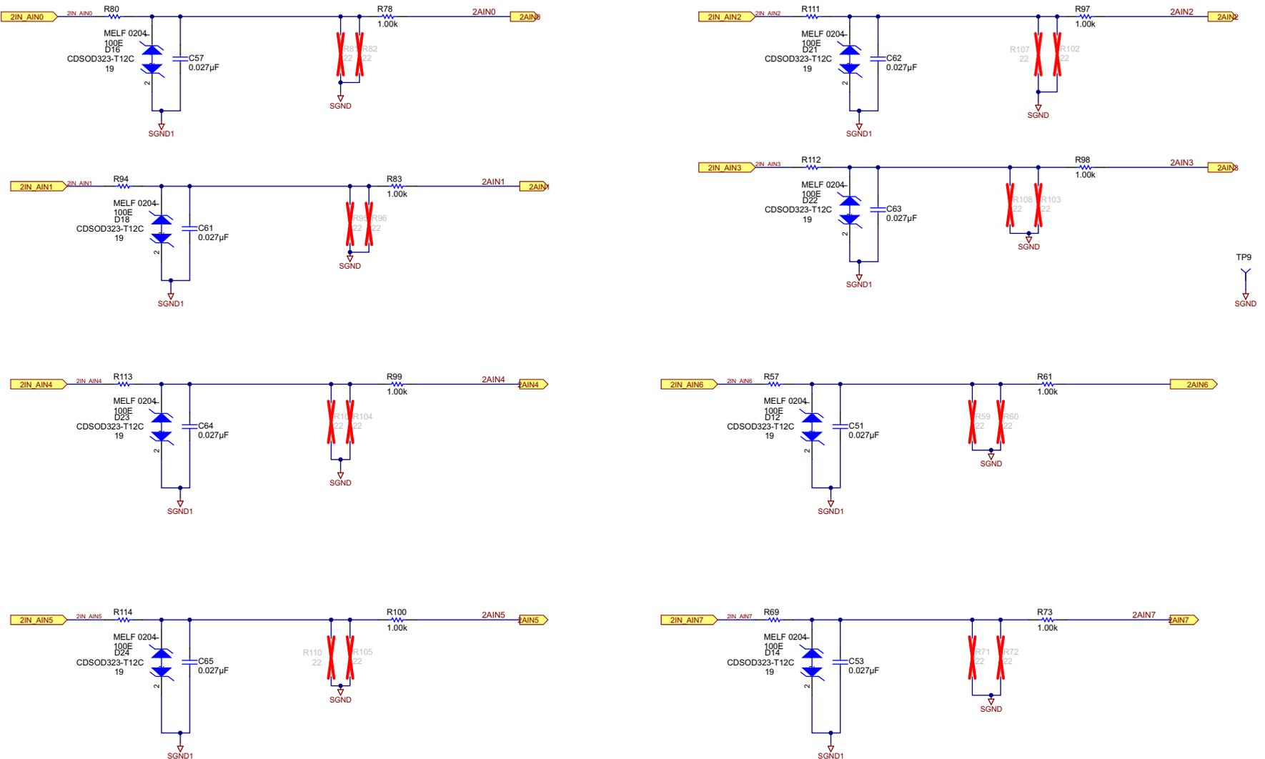
Figure 32. ADC<sub>2</sub> Filters Schematic
