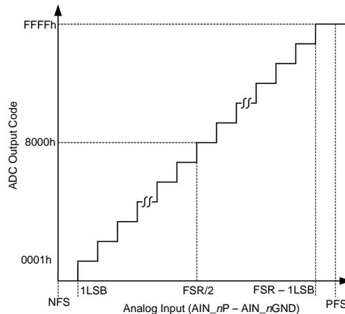
Figure 17. 16-Bit ADC Transfer Function (Straight Binary Format)
