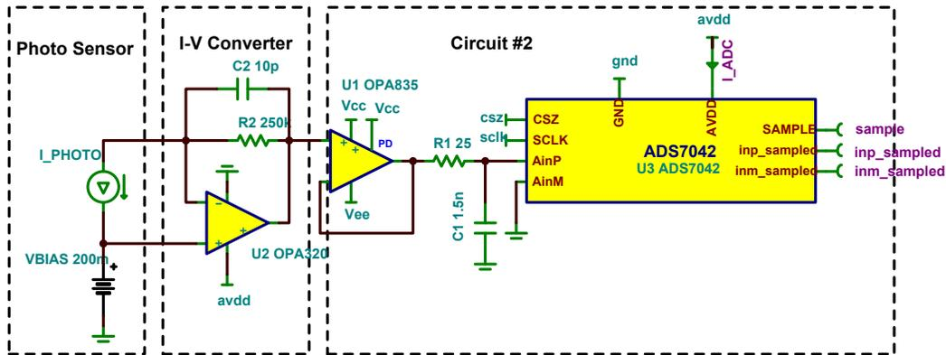
Figure 33: Application Example Using Circuit #2-Photodiode Measurement
