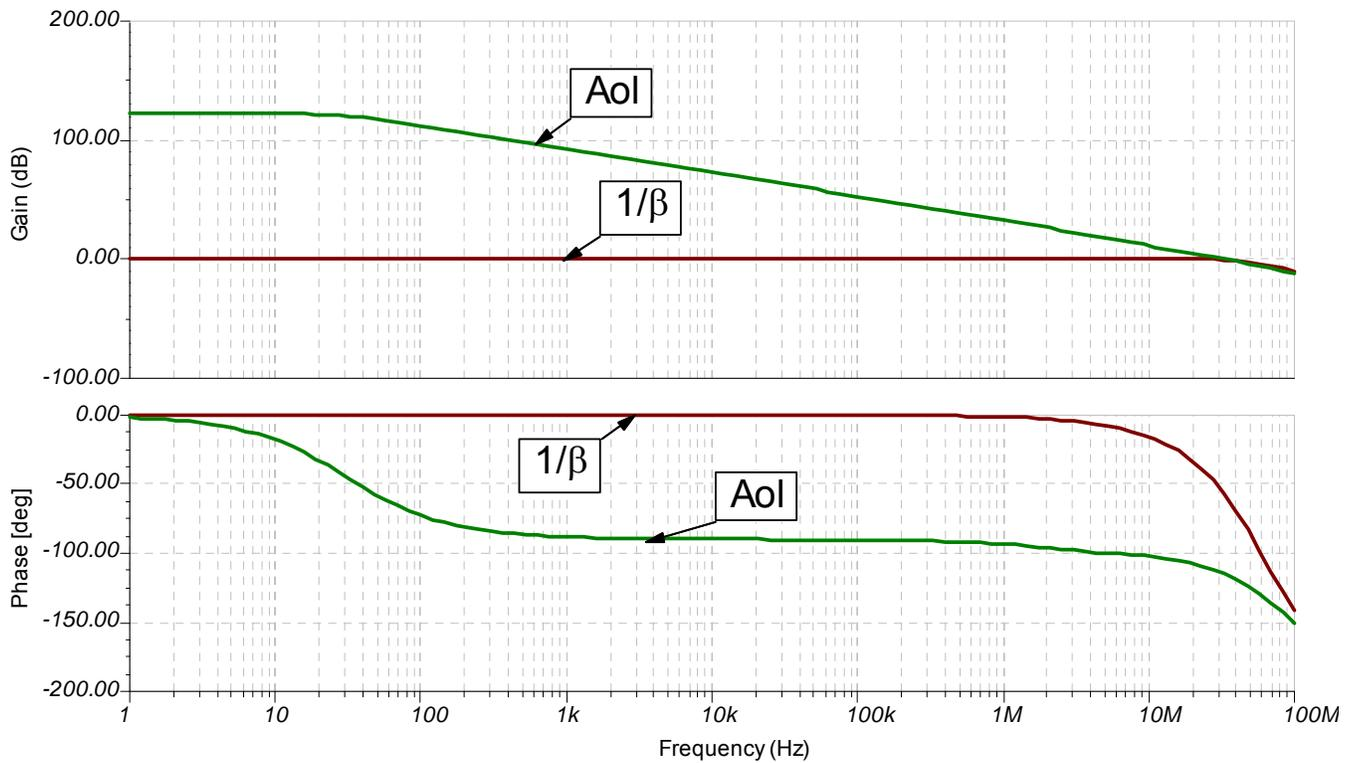
Figure 19: TINA-TI schematic result: AC transfer characteristics for design #2
