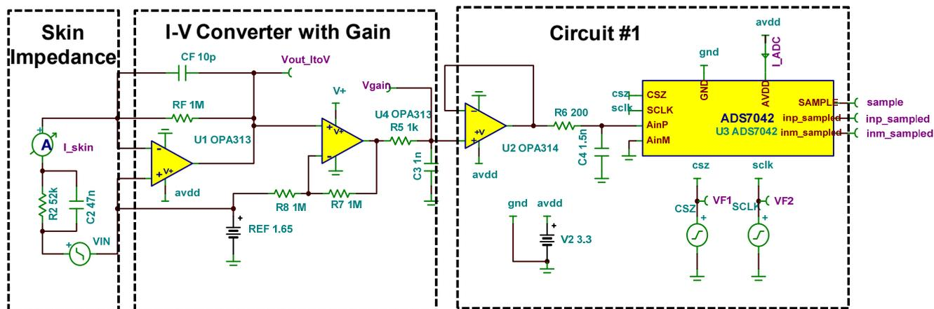
Figure 32: Application Example Using Circuit #2-Skin Impedance Measurement
