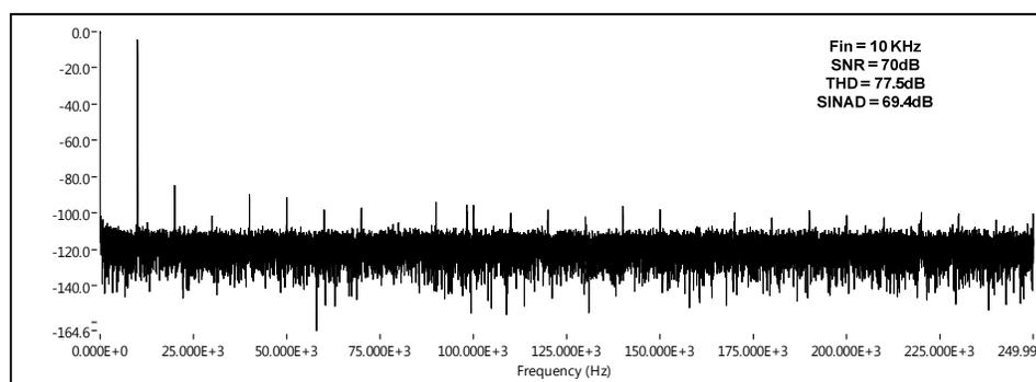
**Figure 1: Measured FFT of a 10 kHz input signal with -0.3dB signal power (Design #1)**
