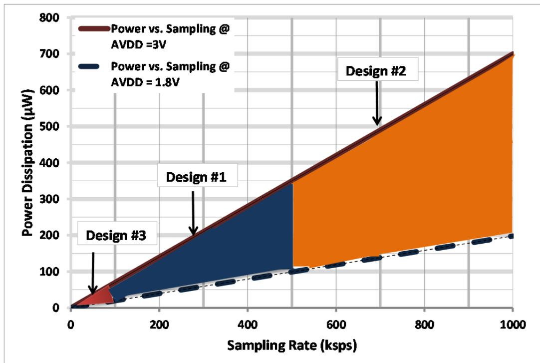
Figure 12: Analog Power Dissipation vs. Sampling Rate (AVDD = 3.3V and 1.8V)
