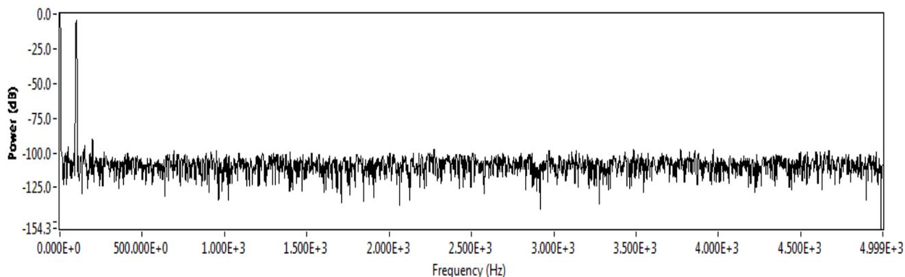
**Figure 3: Measured FFT of a 100Hz input signal with -0.3 dB signal power at 1ksps (Design #3)**
