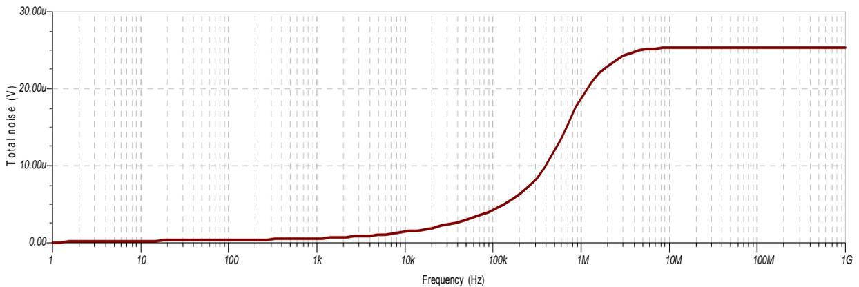
Figure 23: TINA-TI schematic result: Total noise from the driver amplifier for design #1
