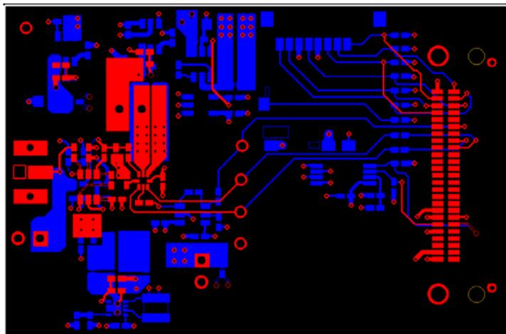
**Figure 29: PCB Layout for ADS7042 Test Board**
