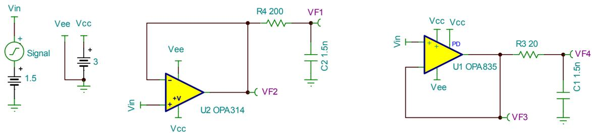
**Figure 20: TINA-TI – Schematic for step response and noise simulation**
