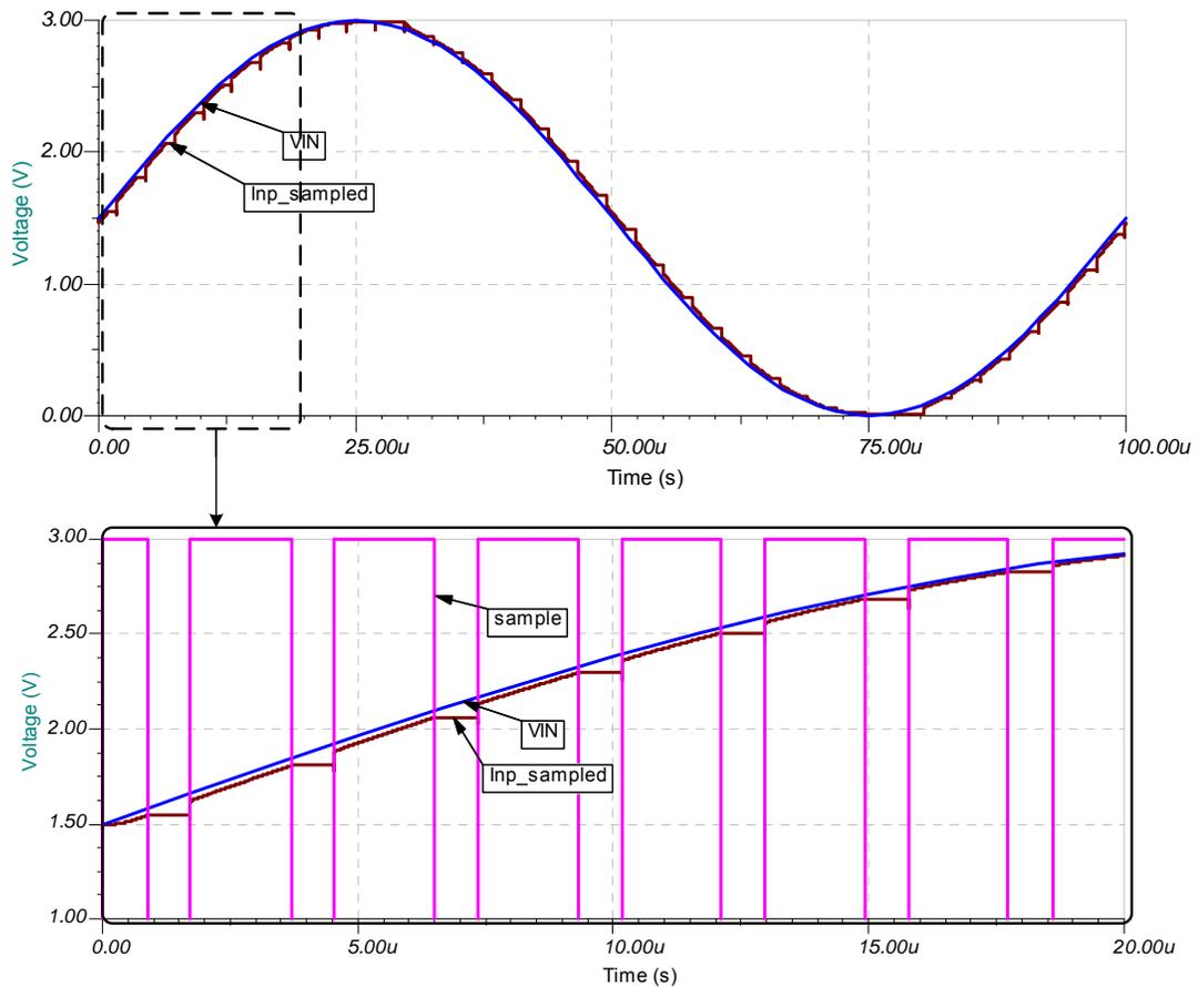
Figure 27: TINA-TI Schematic simulation result: settling of a 10 kHz input signal for design #1
