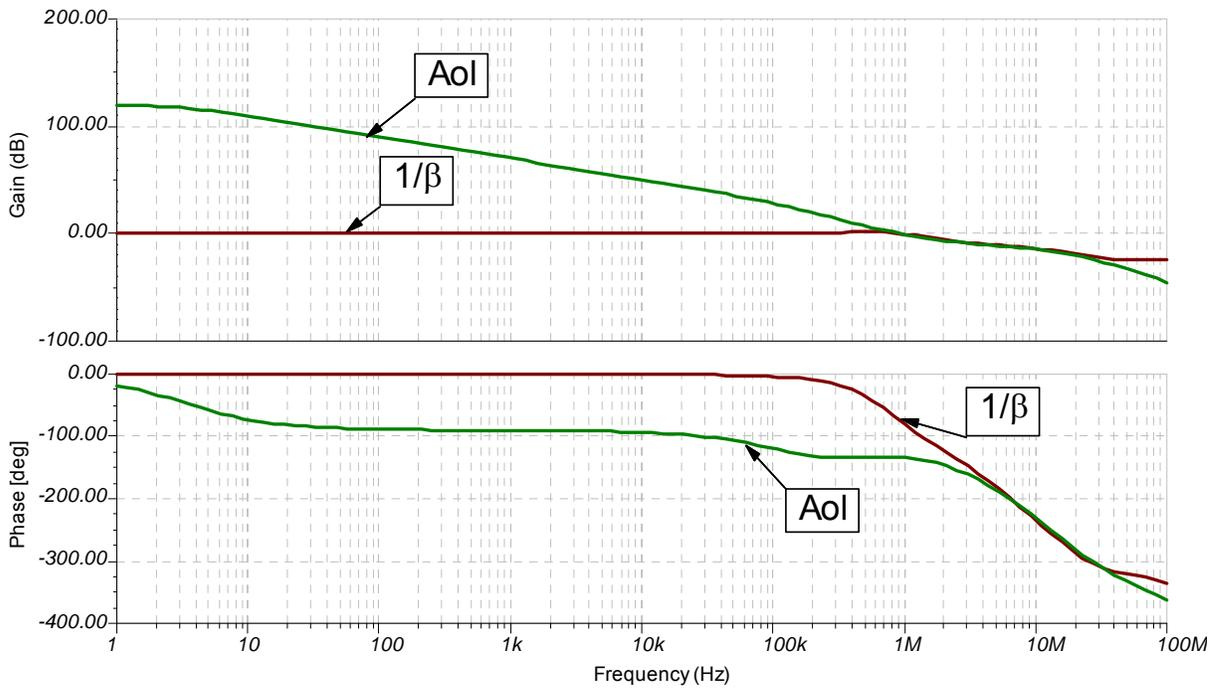
Figure 18: TINA-TI schematic result: AC transfer characteristics for design #1
