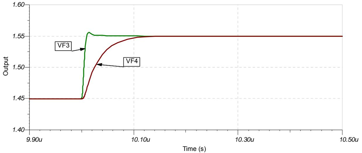
Figure 22: TINA-TI schematic result: Small signal step response for design #2
