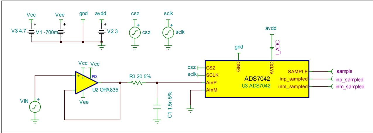
Figure 26: TINA-TI – Schematic for transient response of the track and hold circuit for design #2
