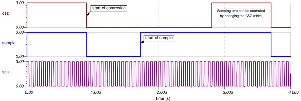
Figure 24: TINA-TI schematic result: ADS7042 timing diagram
