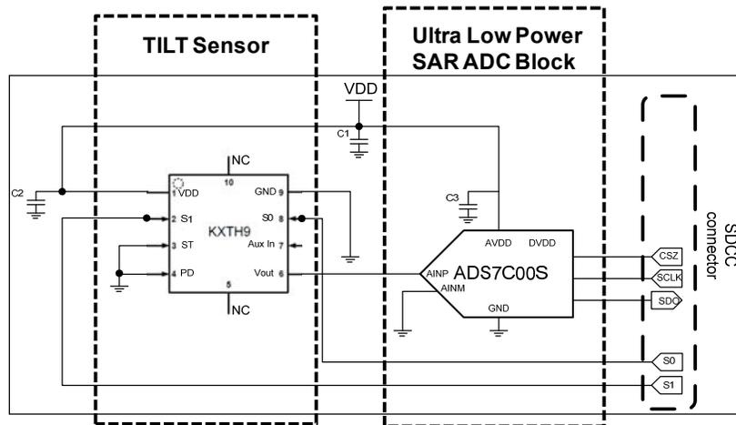
Figure 34: Application Example Using Circuit #3 for a Tilt Sensor Measurement
