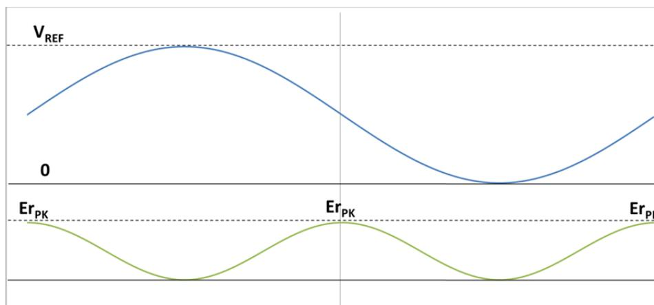
**Figure 7: Plot showing variation of ADC Input Settling Error as Function of ADC Input Signal**
