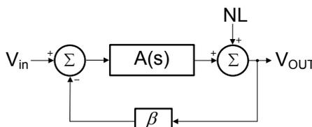
**Figure 5: Transfer Function of a Driver Amplifier with Negative Feedback**
