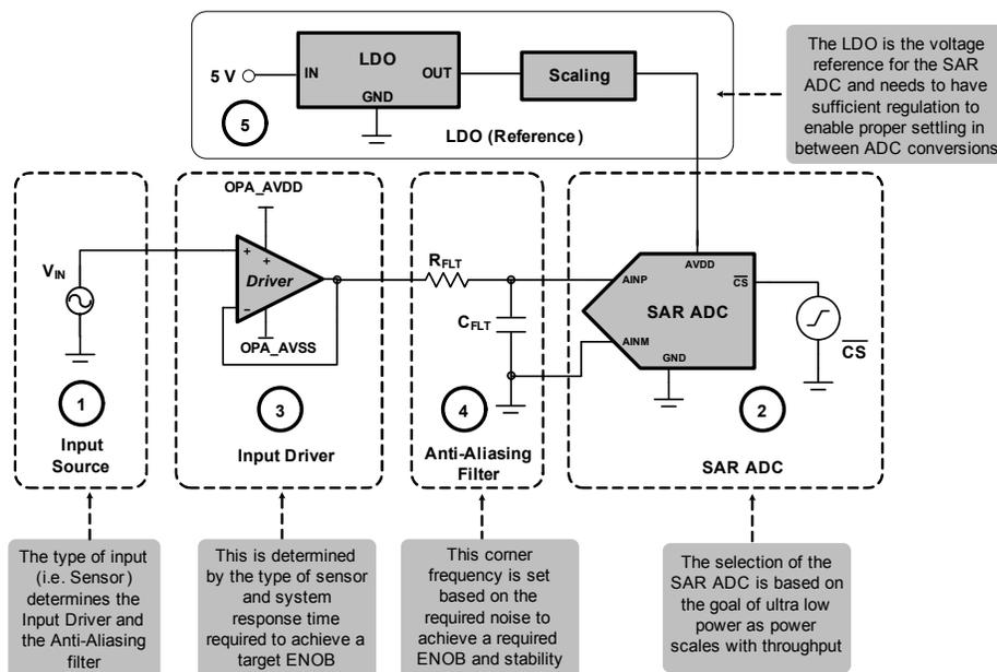
Figure 4: Block Level View of Low Power Data Acquisition Design Steps
