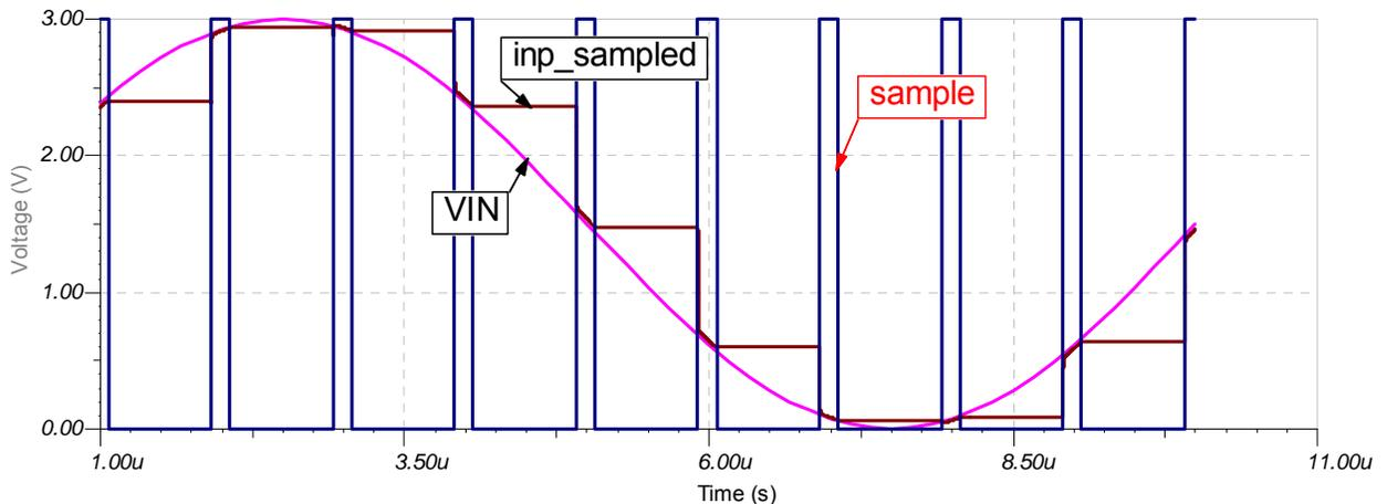
**Figure 28: TINA-TI Schematic simulation result: settling of a 10 kHz input signal for design #2**
