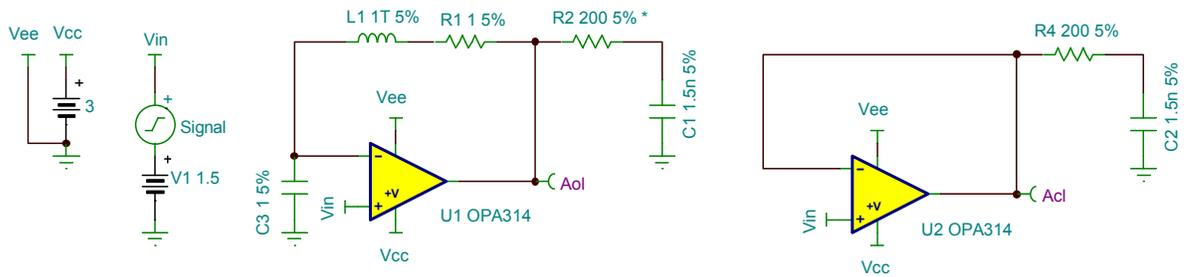
Figure 15: TINA-TI Simulation Circuits for Input Drivers for Designs #1
