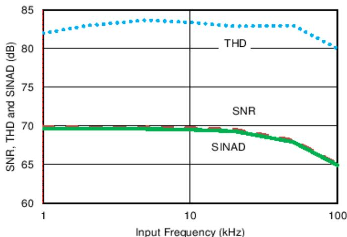
**Figure 30: Dynamic Performance of the OPA835 with Frequency**
