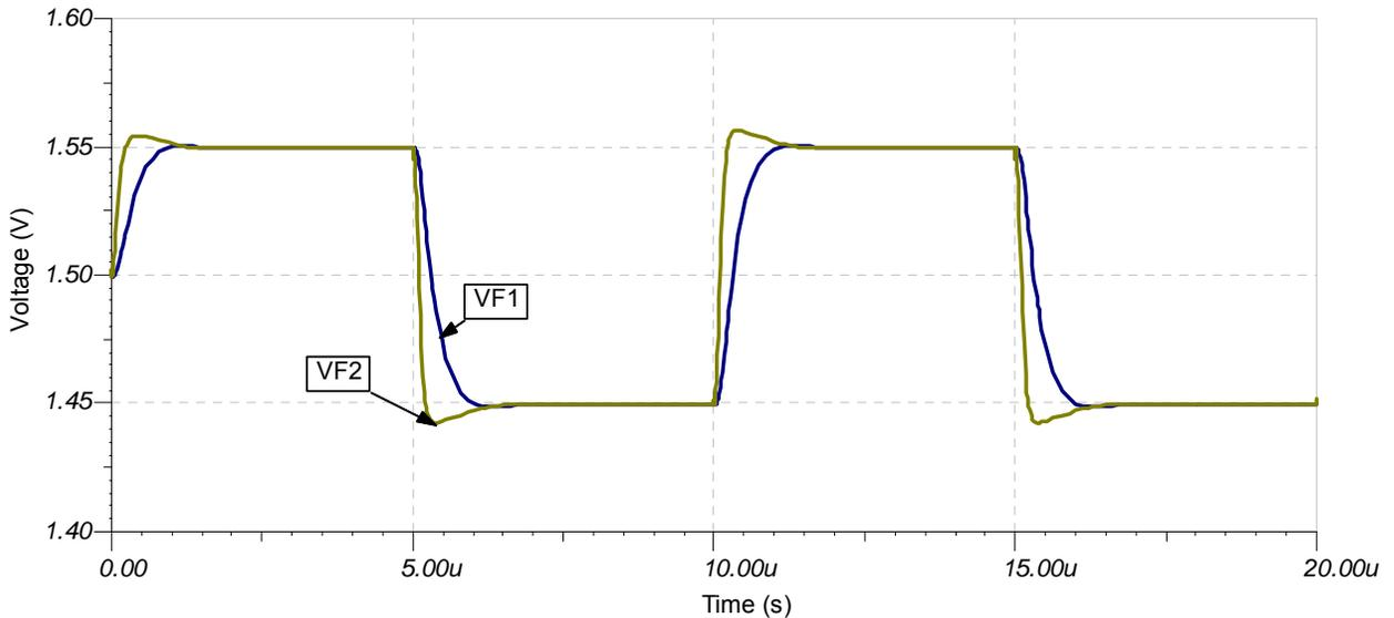
**Figure 21: TINA-TI schematic result: Small signal step response for design #1**
