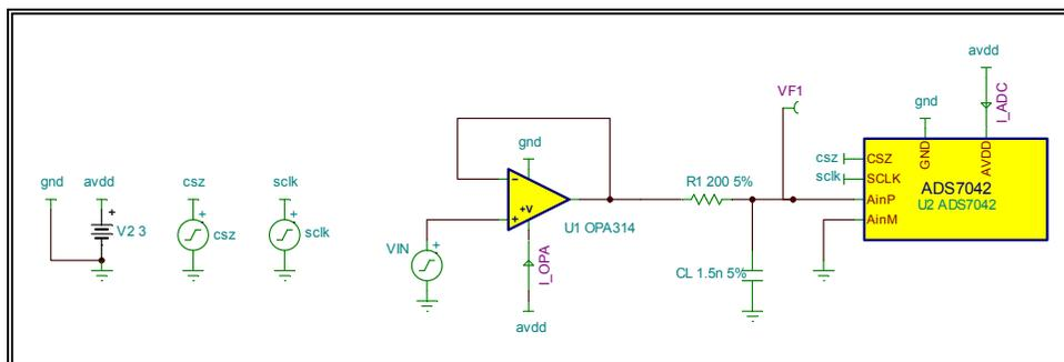
Figure 25: TINA-TI – Schematic for transient response of the track and hold circuit for design #1
