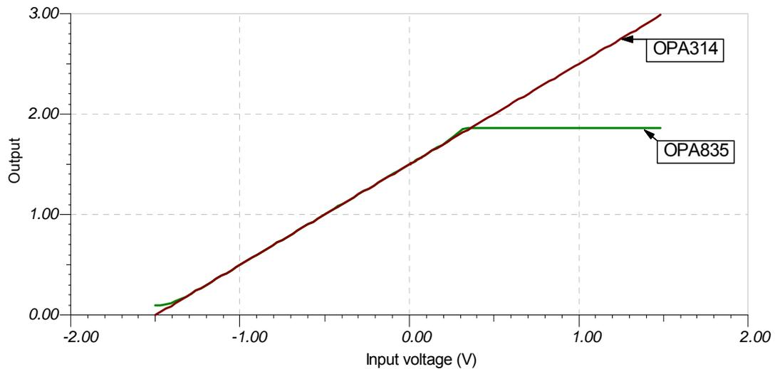
Figure 17: DC Transfer Curve for Design #1 (OPA314) and Design #2 (OPA835)
