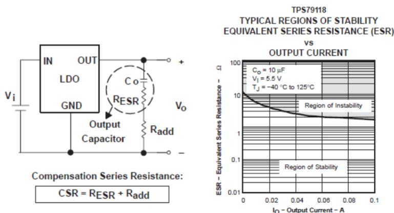
**Figure 10: Diagram Showing Effect of Series Resistance on Stability**
