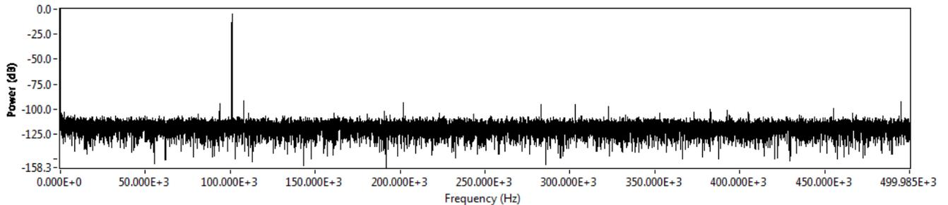
**Figure 2: Measured FFT of a 100 KHz input signal with -0.3 dB signal power (Design #2)**
