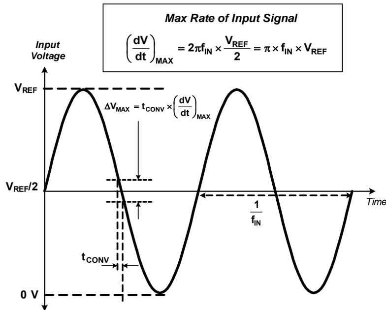
**Figure 8. Analyzing Maximum Change in ADC Input for Sinewave Signal**
