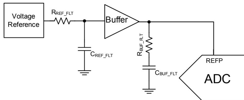
**Figure 9: Simplified Diagram of Voltage Reference and Driver**
