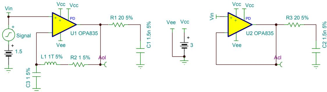
Figure 16: TINA-TI Simulation Circuits for Input Drivers for Designs #2
