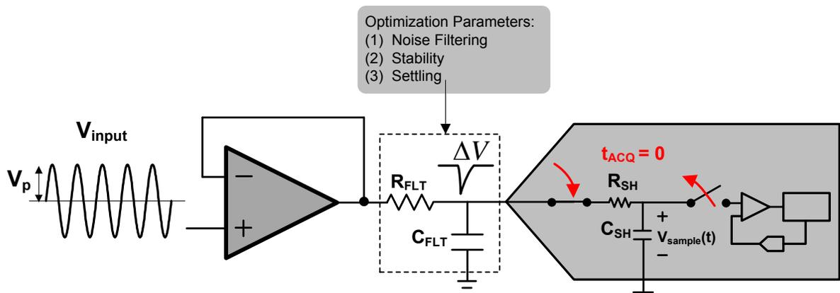
Figure 6. Input Settling Behavior of ADC for Sinusoidal Signal
