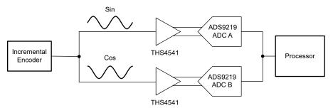
Figure 3. Encoder block diagram with THS device
