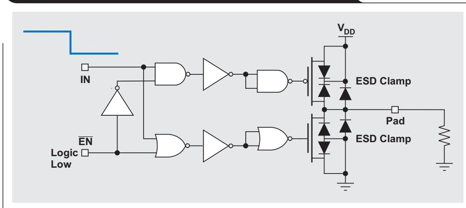
Figure 3 shows the proper test-circuit configuration for the transient falling edge of an output buffer. The resistor following the pad is usually 50 Ω; however, it can be a different value depending on the IC's requirements as stated in the product data sheet.
