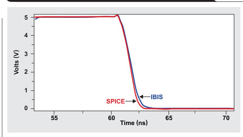
Figure 8 shows a similar fall-time comparison between the SPICE and IBIS models, also based on the ADS8319. Simulated model conditions were based on a 5-V power supply, a junction temperature of 25°C, and a typical process corner.
