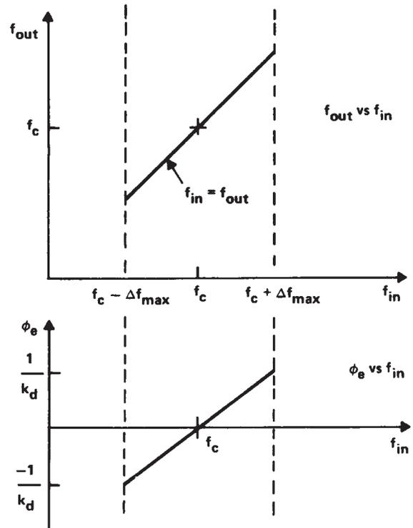
Figure 4. DPLL Transfer Characteristics (in lock)
