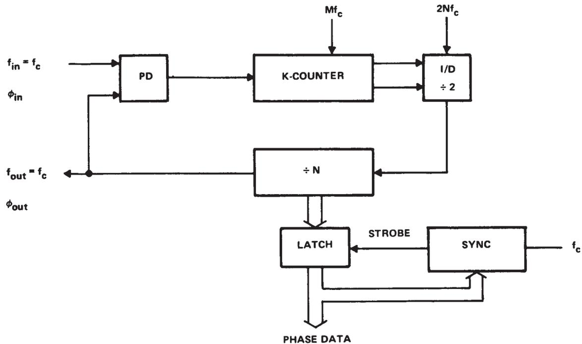
Figure 11. Phase-Shift Demodulator
