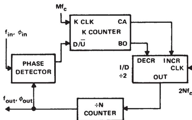
Figure 1. First Order Digital Phase-Locked Loop
