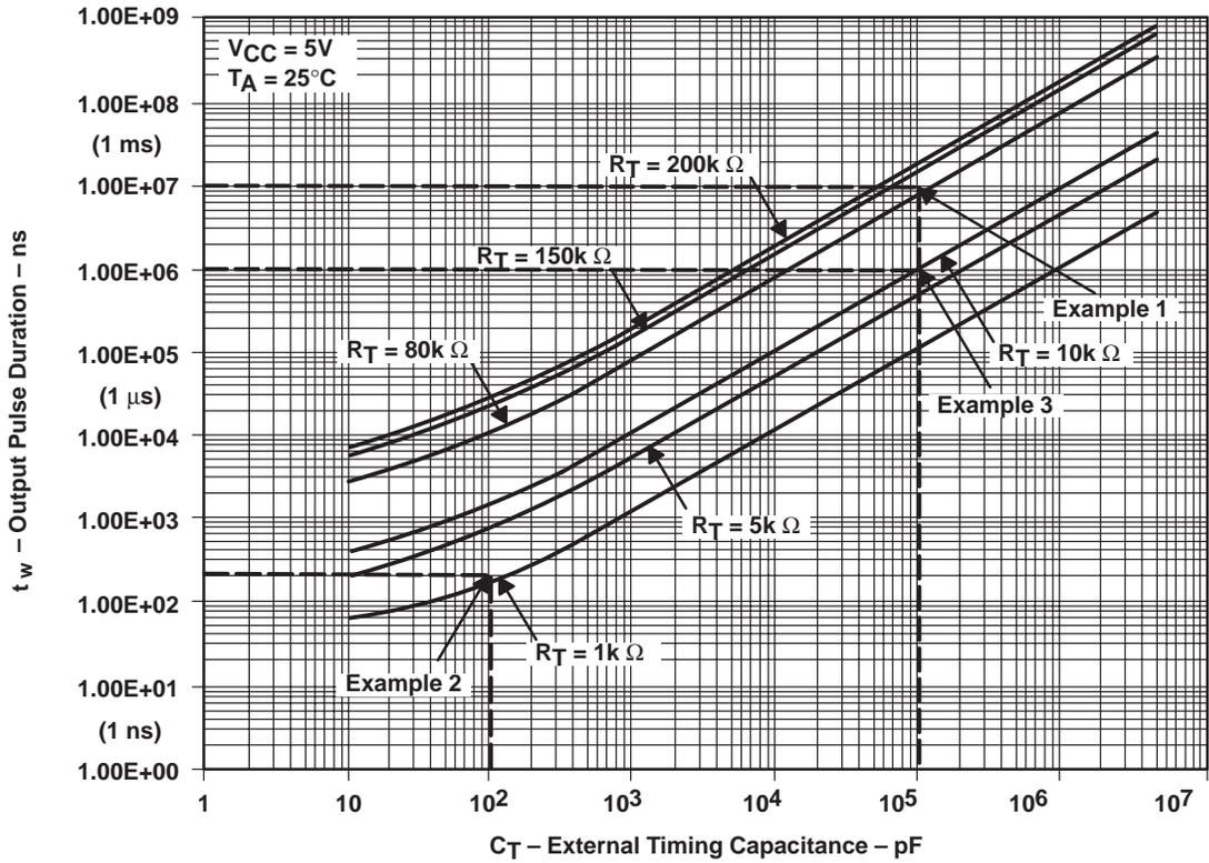
Figure 3. Output Pulse Duration vs External Timing Capacitance
