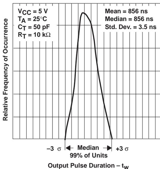
Figure 8. Distribution of Units vs Output Pulse Duration
