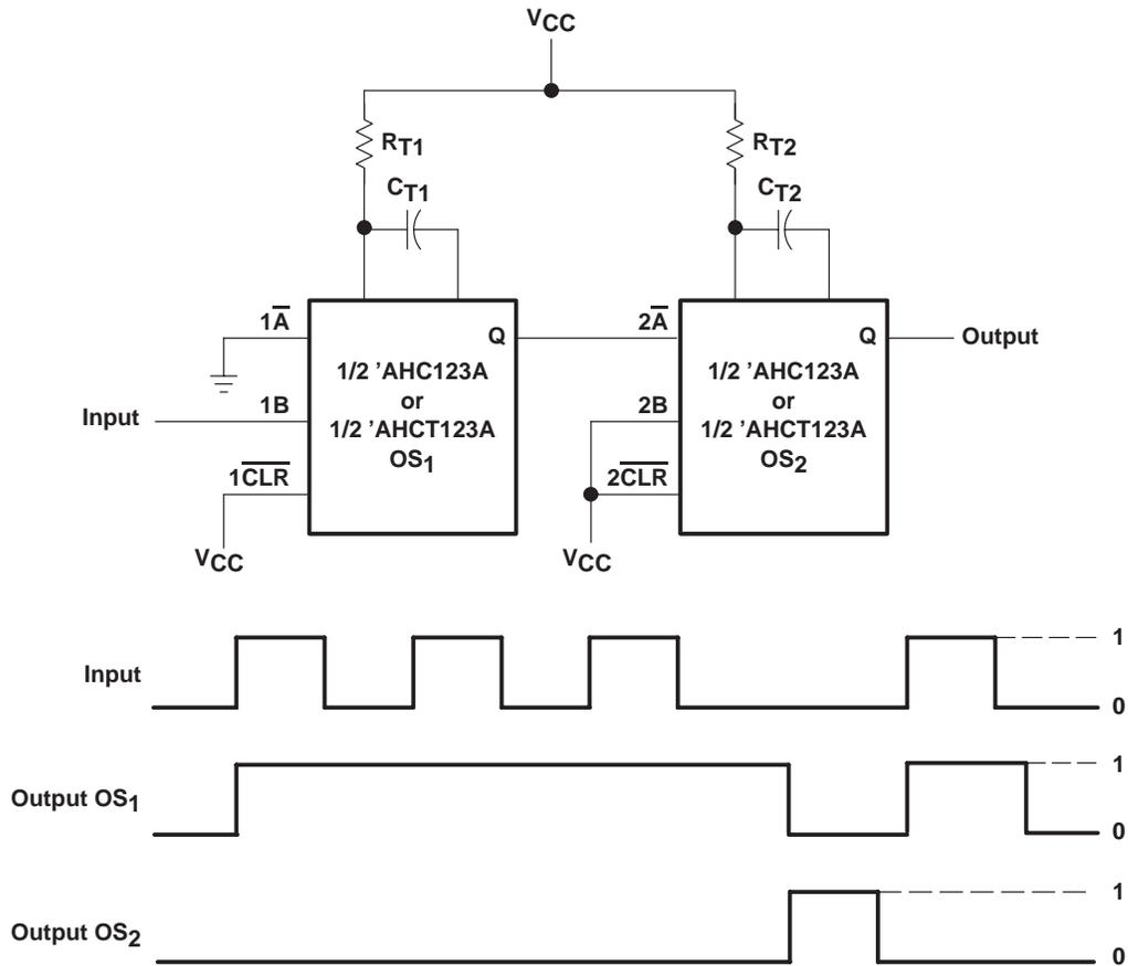
Figure 10. Missing-Pulse Detector
