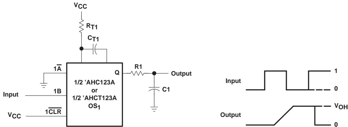
Figure 14. Frequency-Discriminator Circuit
