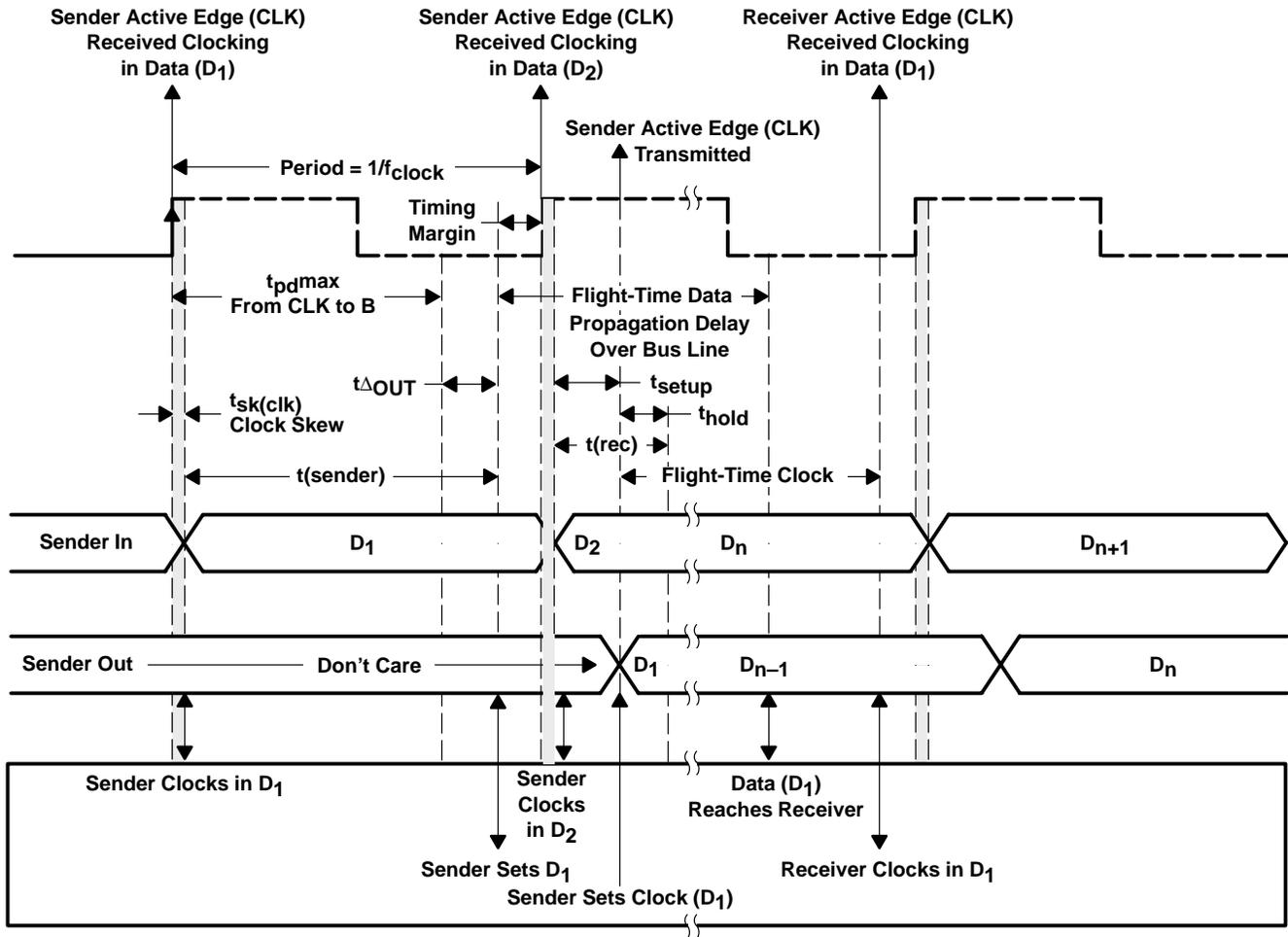
**Figure 13. Time Budget for Source-Synchronous Clock Distribution**
