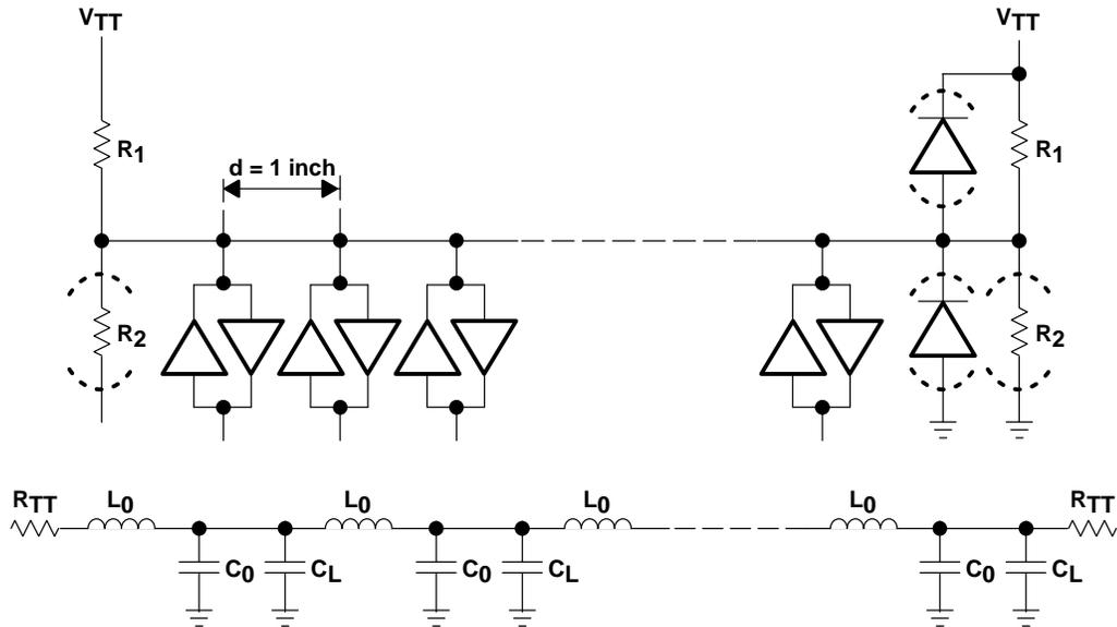
**Figure 2. Additional Capacitive Load of Line by Modules**
