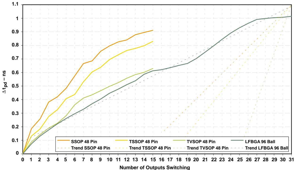
**Figure 7. Effect of Simultaneous Switching on Propagation Time**
