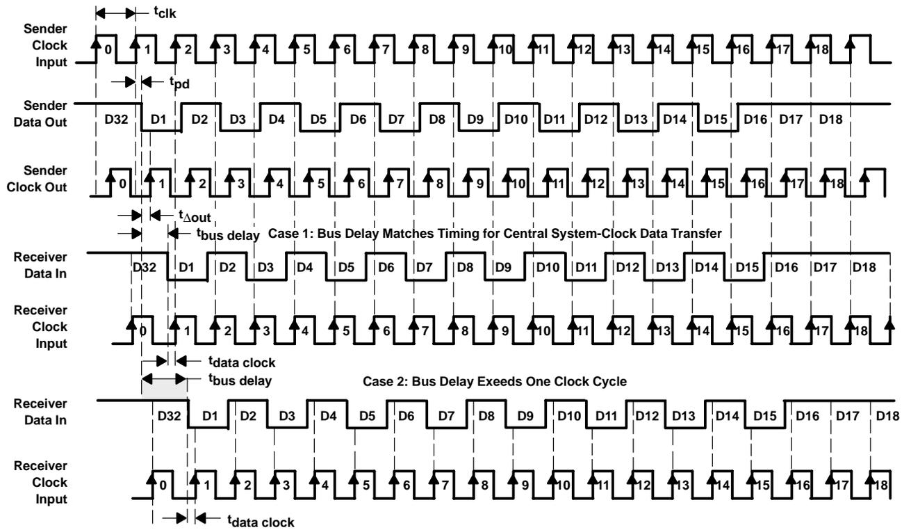
Figure 14. Two Examples of Source-Synchronous Clock Distribution
