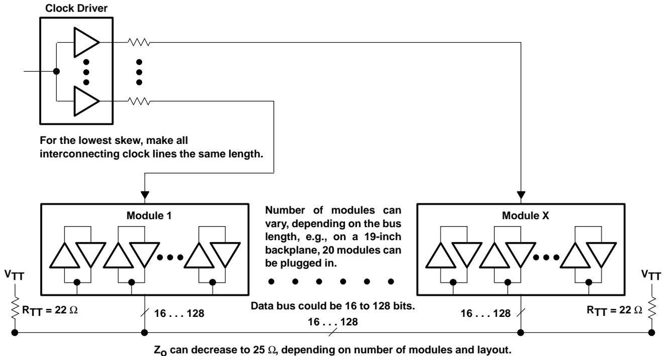
**Figure 9. Principle of Central Synchronous Clock Distribution**
