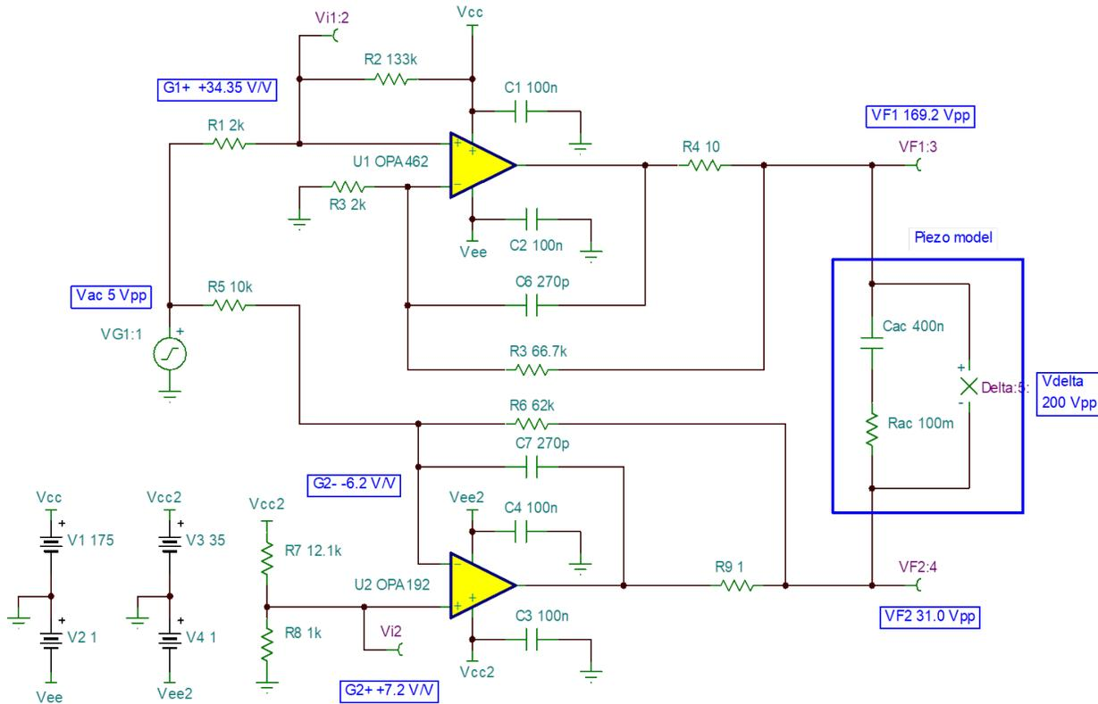
Figure 2-1. Schematic for 200-V Bridged-Output Piezo Driver
