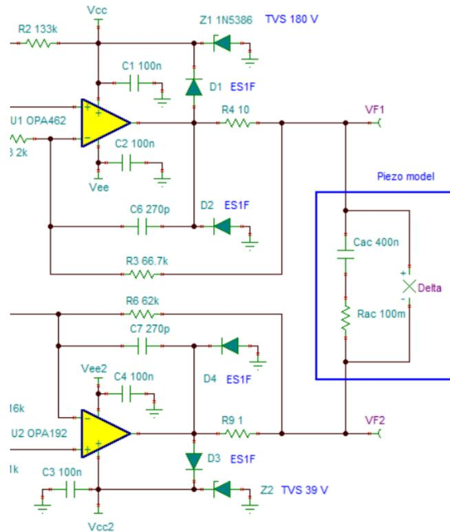
Figure 2-3. Fast Rectifier Diodes D1 – D4 and TVS Diodes Z1 and Z2 Added to Protect U1 and U2 Outputs
