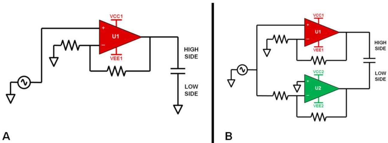
**Figure 1-1. Driving a Piezoelectric Load With a Single Amplifier (A) and Bridge Arrangement (B)**
