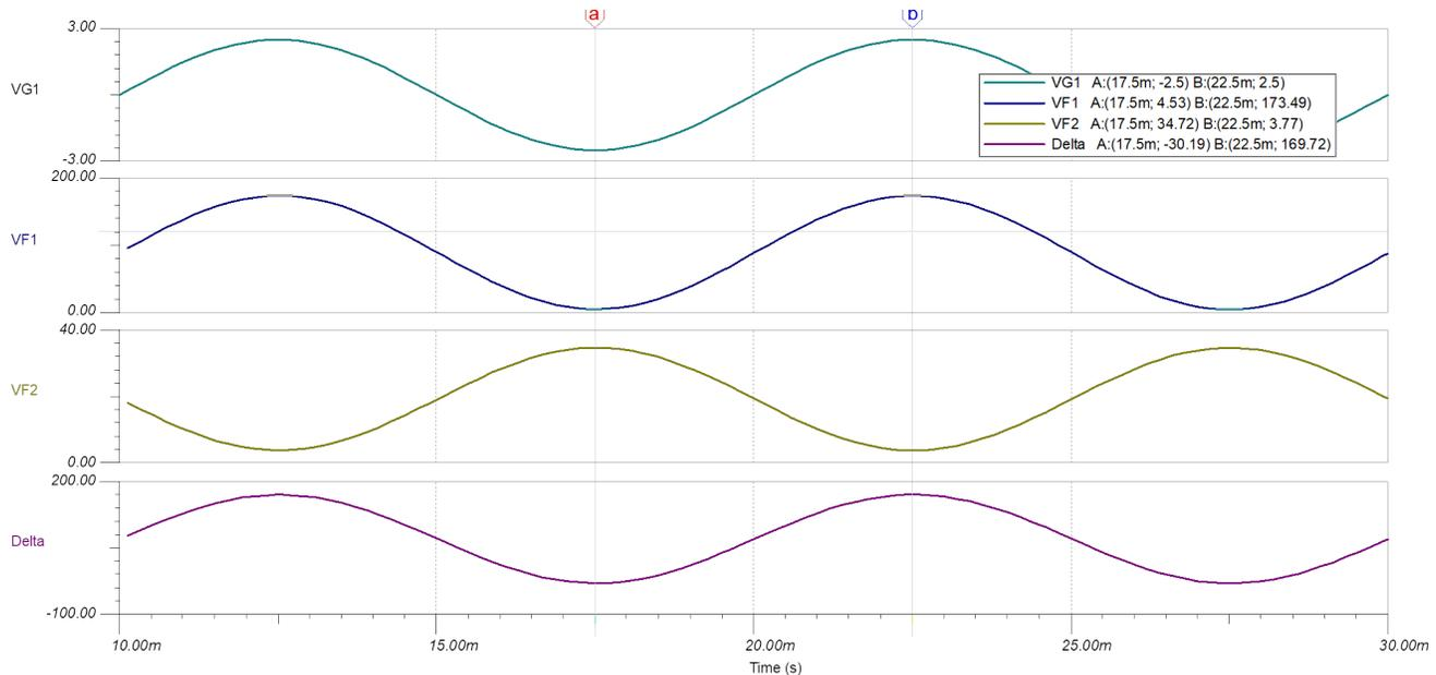
**Figure 2-2. Transient Simulation Results for Bridged Output Circuit With 5-Vpp, 100-Hz Sinusoidal Input**
