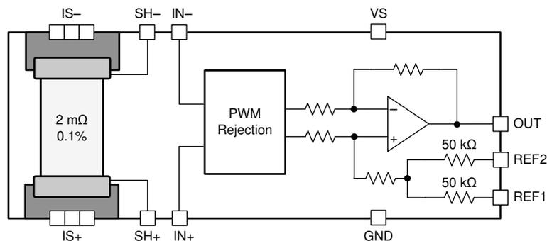
Figure 1-1. Functional Block Diagram
