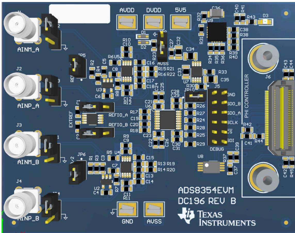
Figure 5-1. ADS8354EVM-PDK Jumper Locations
