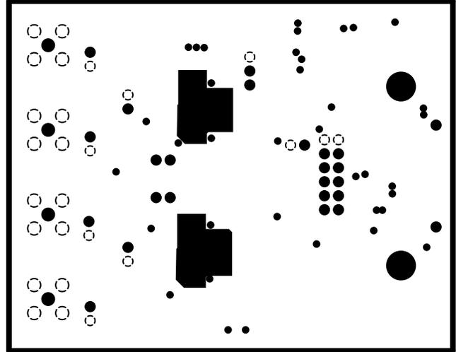
Figure 7-2. ADS8354EVM PCB Layer 2: GND Plane
