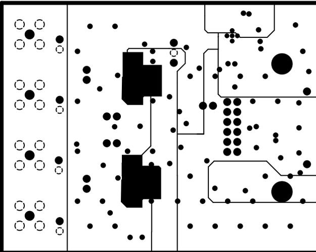
Figure 7-3. ADS8354EVM PCB Layer 3: Power Plane
