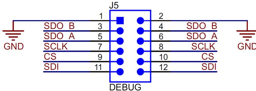
Figure 3-1. ADS8354EVM Debug Header
