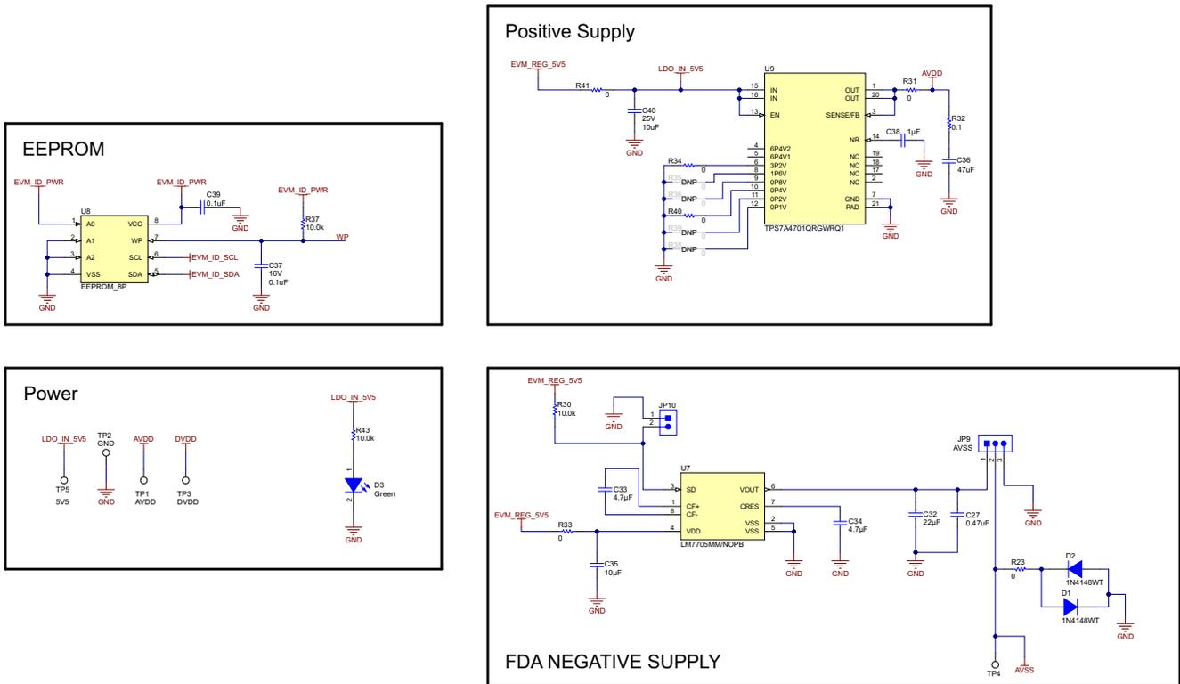
Figure 7-5. Schematic Diagram (Page 1): EEPROM, Power Supplies
