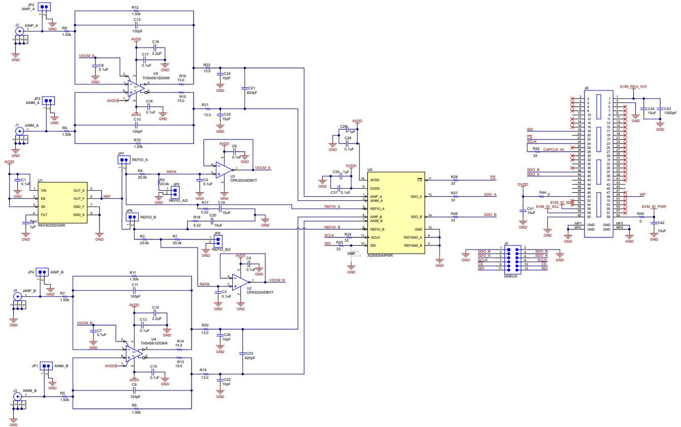
Figure 7-6. Schematic Diagram (Page 2): Analog Inputs, ADC Main, External Reference, PHI Connector
