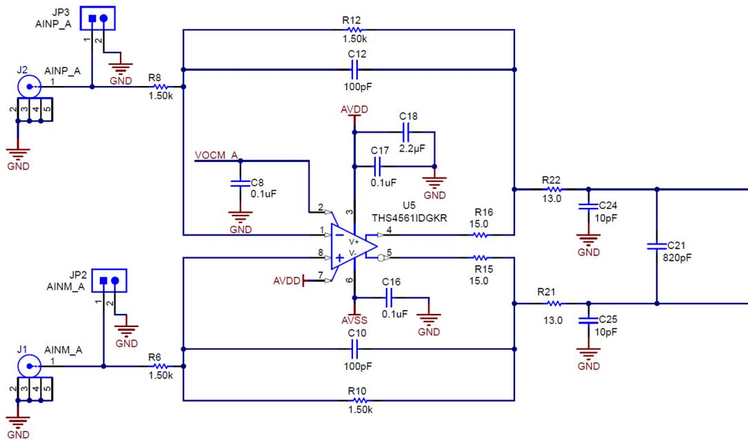
Figure 2-1. ADS8354EVM Analog Input Path
