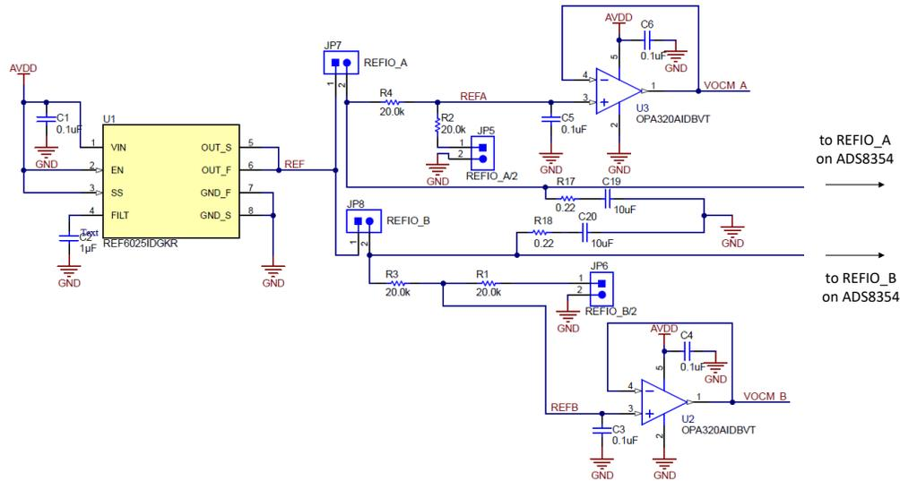
Figure 2-2. ADS8354EVM Common-Mode Voltage Buffer Circuit
