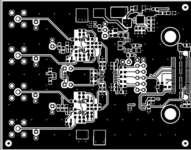
Figure 7-1. ADS8354EVM PCB Layer 1: Top Layer
