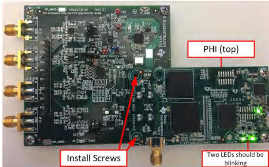
**Figure 6-1. ADS8332EVMV2-PDK Hardware Setup and LED Indicators**
