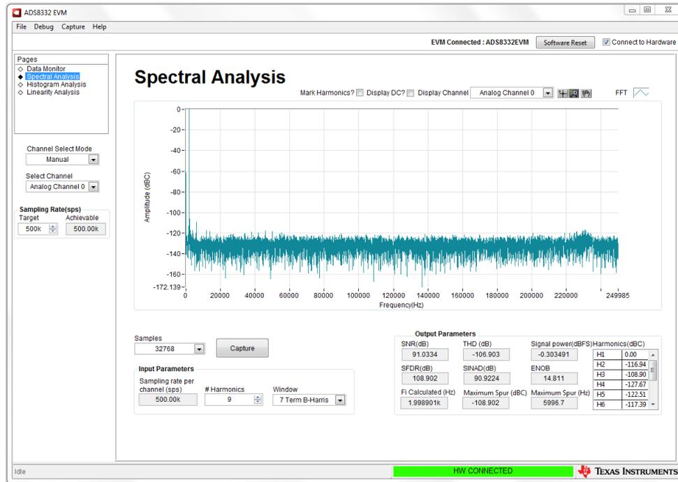
Figure 6-6. Spectral Analysis Tool
