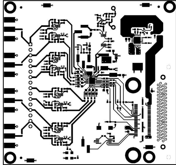
Figure 7-2. ADS8332EVMV2 PCB Layer 1: Top Layer
