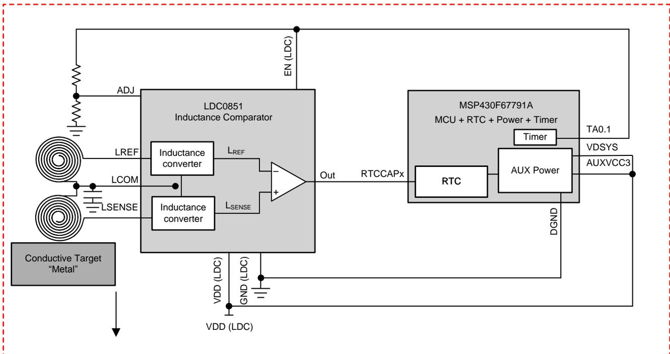
shows the block diagram of this one-sense-coil variant.
