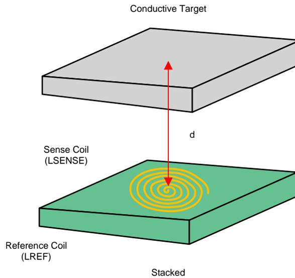
**Figure 15. Stacked Coil Solution Type**
