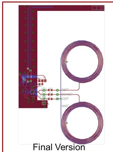
**Fig. 28. Coil Implemented in Design**
