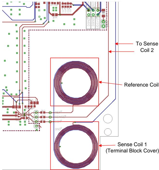
図 32. Reference and Sense Coil 1 of Two-Sense-Coil Implementation
