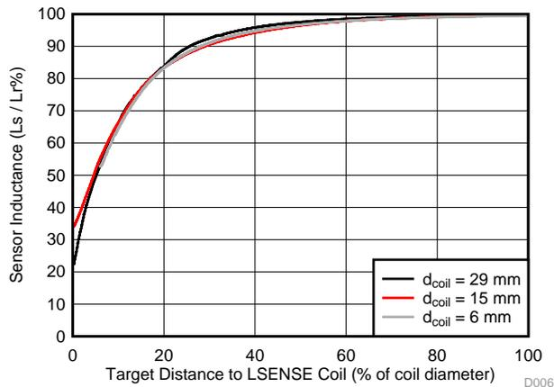
**図 7. Sensor Inductance versus Target Distance**
