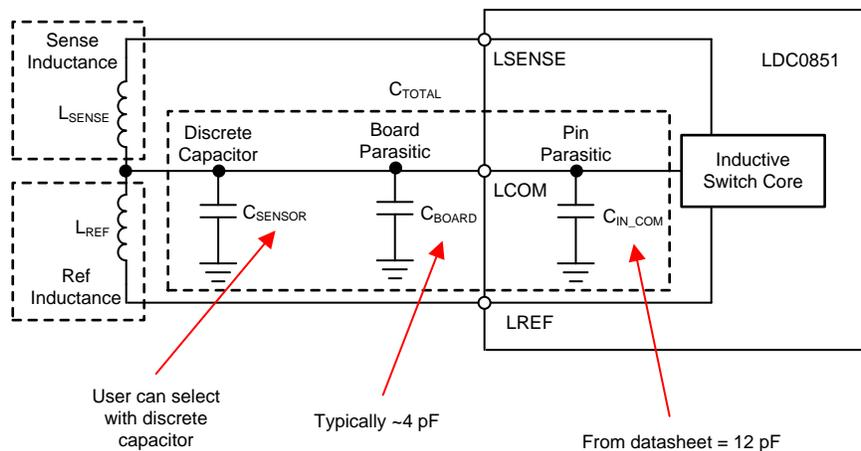
図 9. LDC0851 Sensing Components
