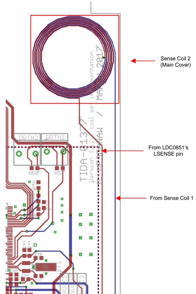
図 33. Sense Coil 2 of Two-Sense-Coil Implementation
