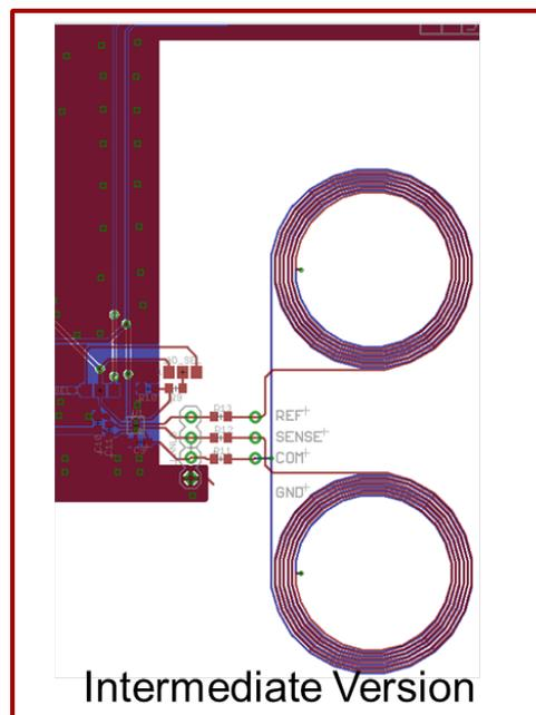
図 27. First Modifications Made to WEBENCH Coil
