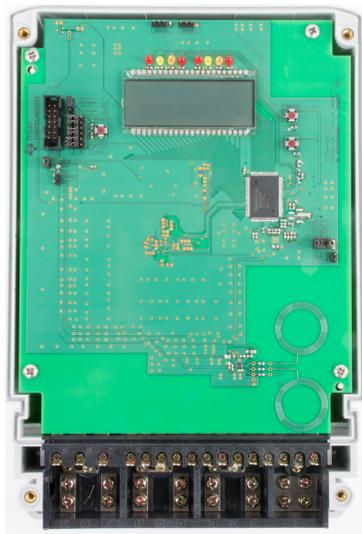
**Figure 43. TIDA-01377 PCB One-Sense-Coil Variant Top View**
