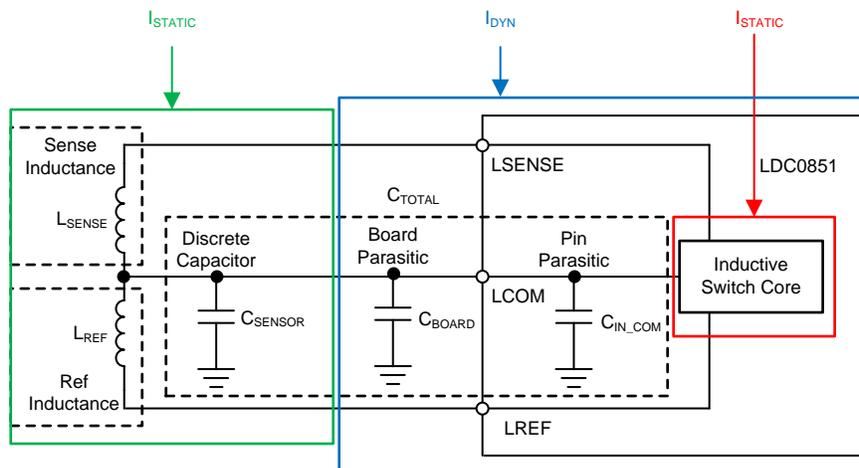
図 36. LDC0851 Active Current Consumption Components
