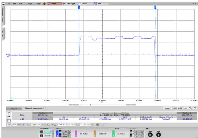
☒ 52. Average Current Consumption: LDC0851 Enabled, Two-Sense-Coil Implementation
