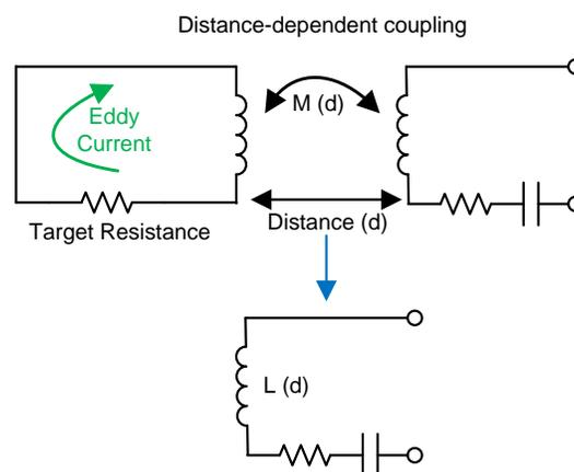
**Figure 6. Electrical Model of Series Inductive Sensor**
