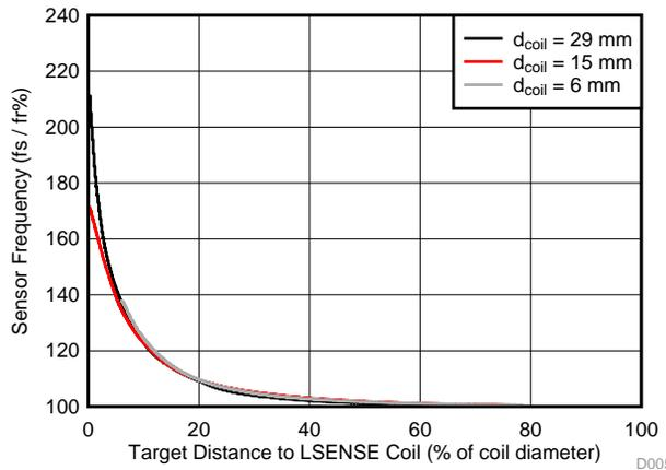
図 8. Sensor Frequency versus Target Distance
