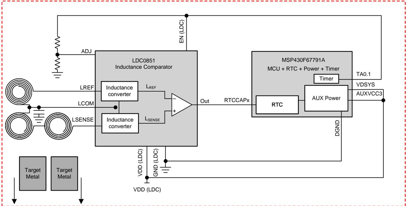
shows the block diagram of the two sense variant of this design.
