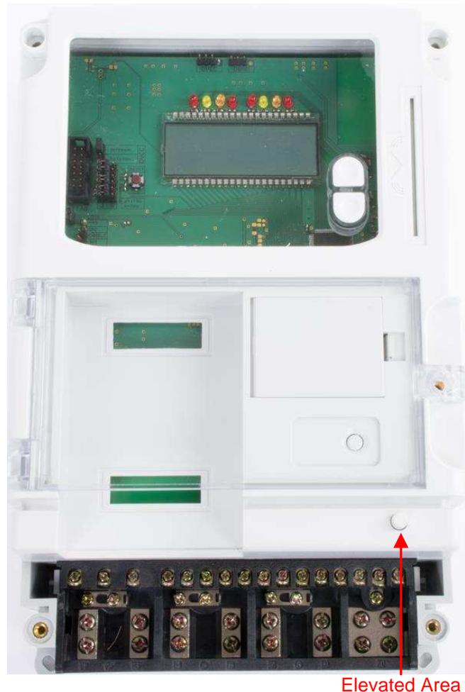
Figure 23. Main Cover Placed on e-Meter Case
