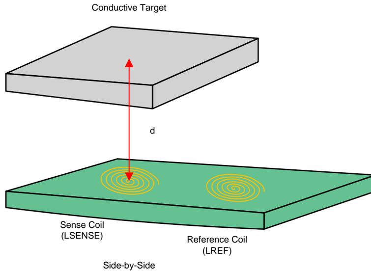
☒ 16. Side-by-Side Coil Solution Type
