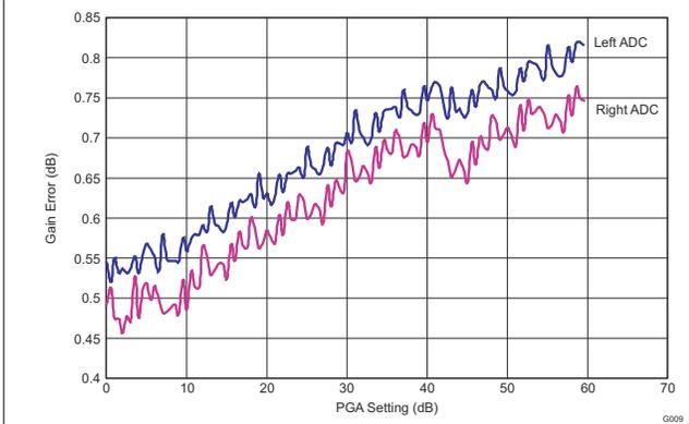
Figure 8-9. ADC Gain Error vs PGA Gain Setting
