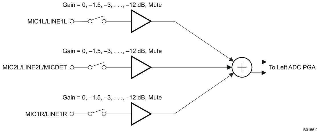
☒ 10-14. Left-Channel, Single-Ended Analog Input Mixing Configuration
