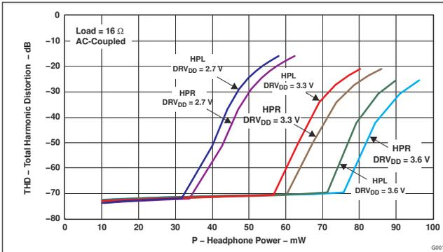
Figure 8-5. THD vs Headphone Power, 16-Ω Load
