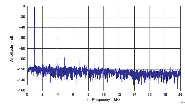
Figure 8-7. Line Input to ADC FFT Plot
