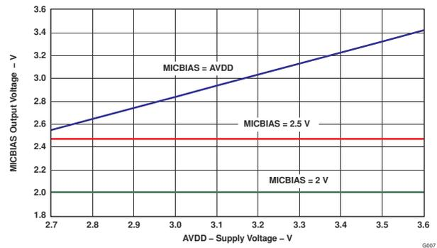
Figure 8-10. MICBIAS Output Voltage vs AVDD
