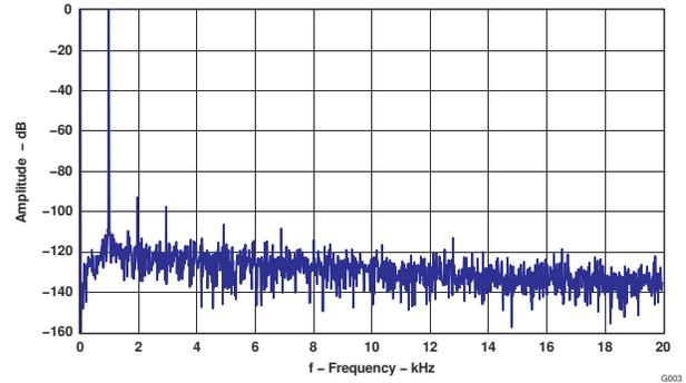
Figure 8-6. DAC to Line Output FFT Plot
