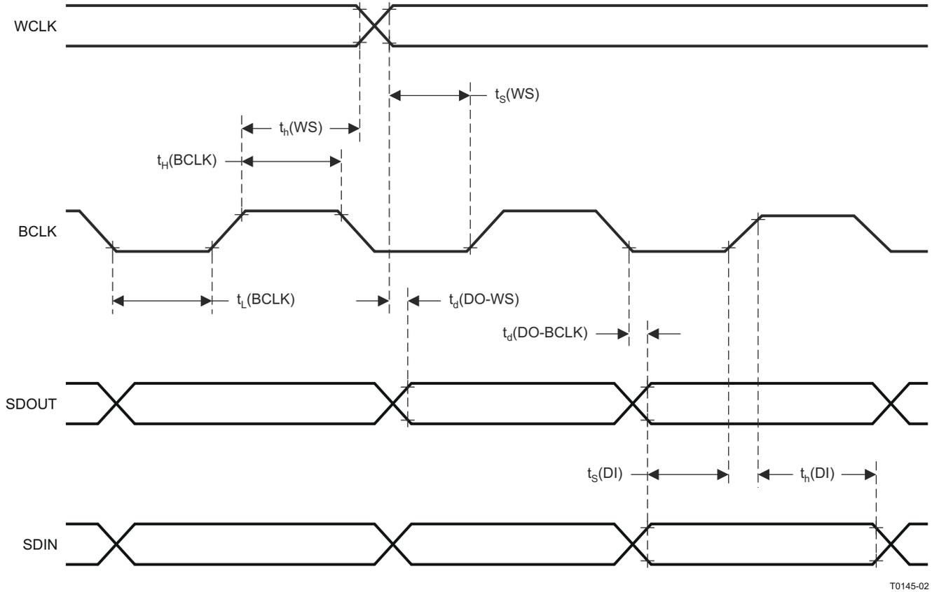
**图 8-3. I2S, L2J, R2J Timing in Slave Mode**
