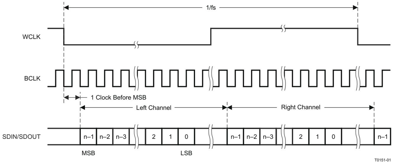
**FIG 10-5. I2S Serial Data Bus Mode Operation**
