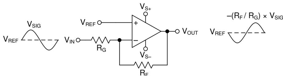
**Figure 7-2. Inverting Amplifier**
