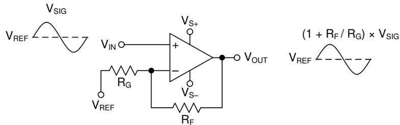
**Figure 7-1. Noninverting Amplifier**
