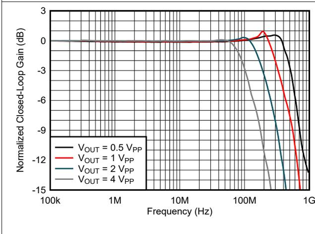
Figure 6-3. Noninverting Large-Signal Frequency Response
