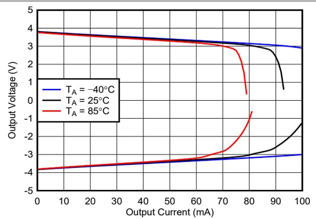
6-26. Output Voltage vs Output Current Over Temperature
