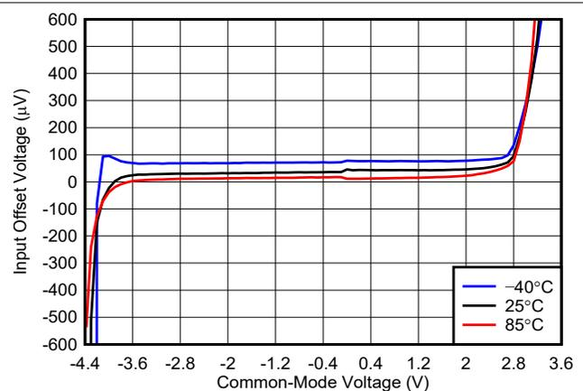
6-30. Input Offset Voltage vs Common-Mode Voltage Over Temperature
