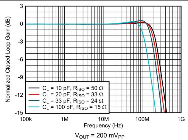
**6-8. Frequency Response vs Capacitive Load**
