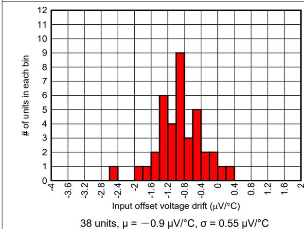
6-29. Input Offset Voltage Drift Histogram
