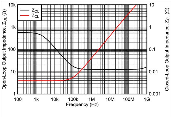
6-24. Open-Loop and Closed-Loop Output Impedance vs Frequency
