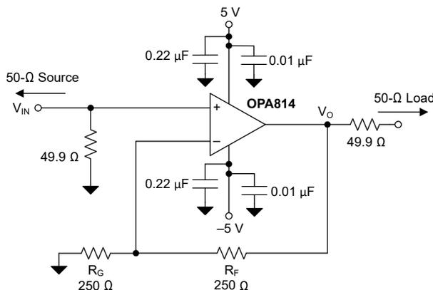
**Figure 8-1. Noninverting  $G = +2$  V/V Configuration and Test Circuit**
