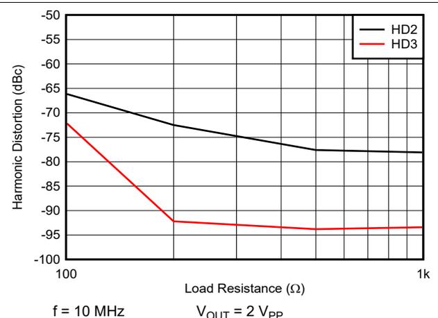
**6-12. Harmonic Distortion vs Load Resistance**
