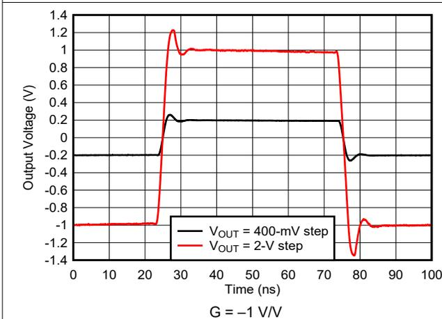
**6-11. Inverting Large-Signal Pulse Response**
