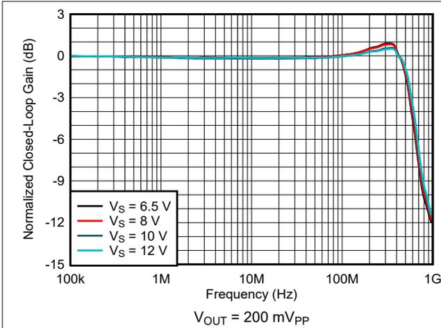
**6-7. Noninverting Small-Signal Frequency Response Over Supply**
