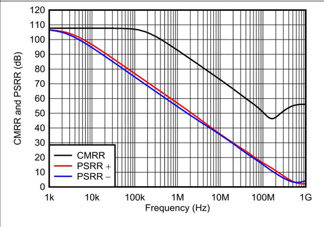
6-22. Common-Mode and Power-Supply Rejection Ratio vs Frequency
