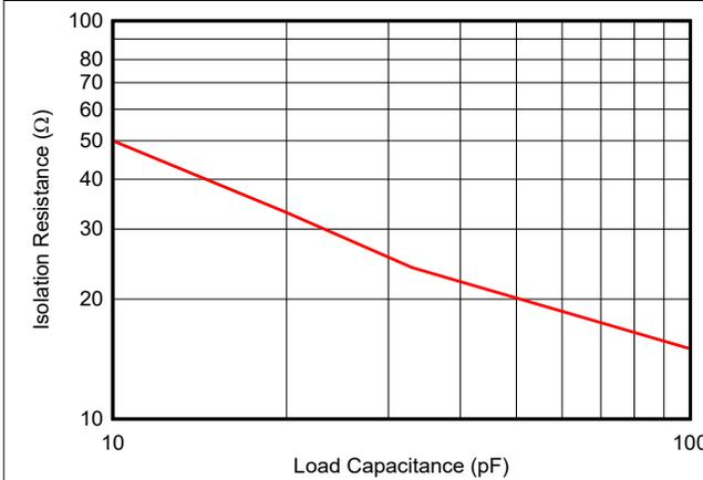
**6-9. Recommended Isolation Resistor vs Capacitive Load**
