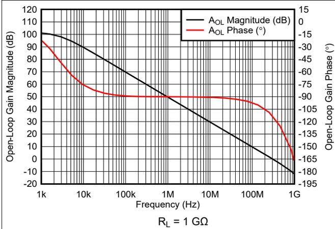
6-23. Open-Loop Gain Magnitude and Phase vs Frequency
