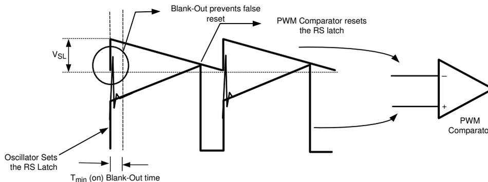
**Figure 6-1. Basic Operation of the PWM Comparator**
