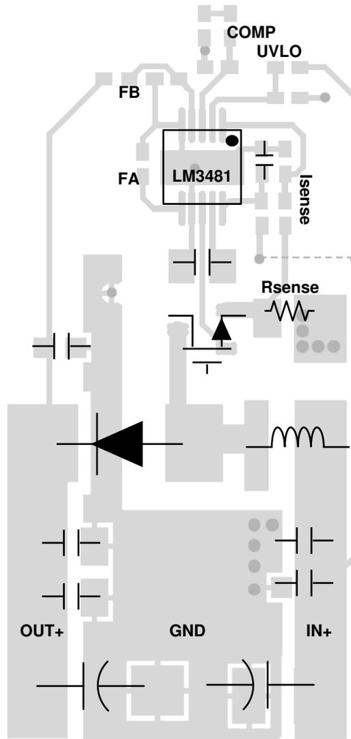
図 7-10. Typical Layout for a Boost Converter
