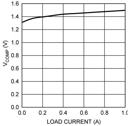
Figure 5-1. Comp Pin Voltage vs. Load Current
