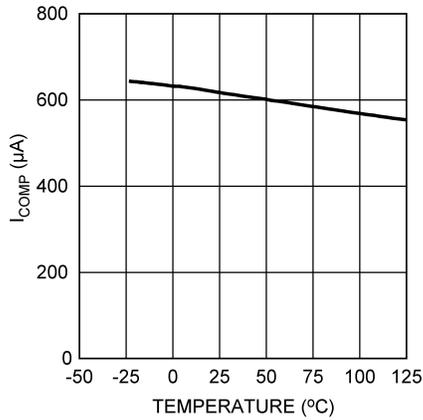
图 5-7. COMP Pin Source Current vs. Temperature
