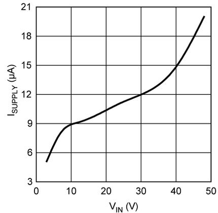
图 5-8. I<sub>SUPPLY</sub> vs. Input Voltage (Nonswitching)
