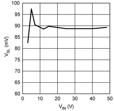
Figure 5-14. Compensation Ramp Amplitude vs. Input Voltage
