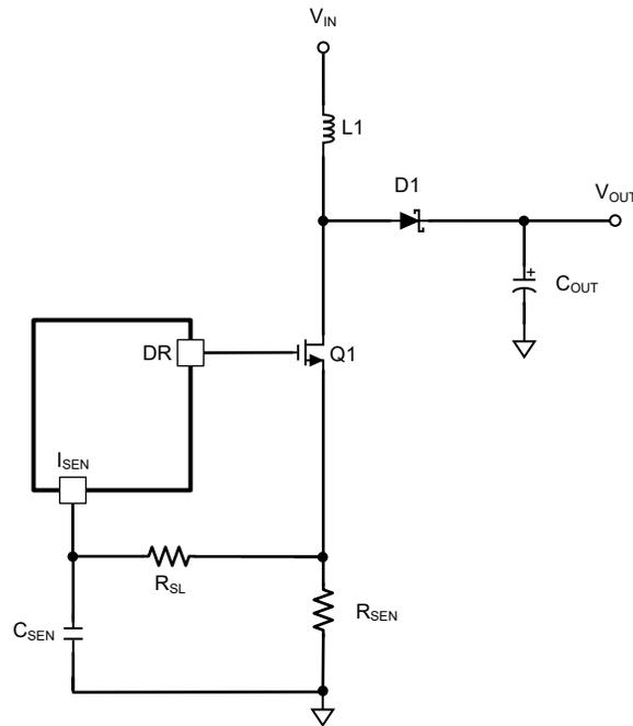
図 6-6. Increasing the Slope of the Compensation Ramp
