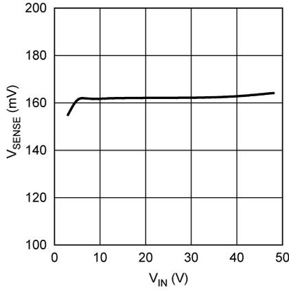
Figure 5-13. Current Sense Threshold vs. Input Voltage
