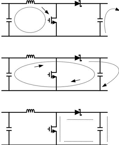
7-9 shows the current flow of a boost converter. The top schematic shows a dotted line which represents the current flow during on-state and the middle schematic shows the current flow during off-state. The bottom schematic shows the currents we refer to as AC currents. These currents are the most critical currents because current is changing in very short time periods. The dotted lined traces of the bottom schematic are the ones to make as short as possible.
