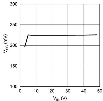
图 5-12. Short Circuit Protection vs. V<sub>IN</sub>
