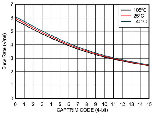
**图 9-2. Output Slew Rate vs. CAPTRIM Code**
