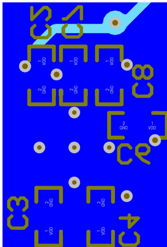
图 11-3. PCB Layout Example for CDCDB400, Bottom Layer
