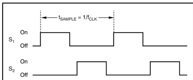
Figure 40. Timing for the Switches in Figure 39
